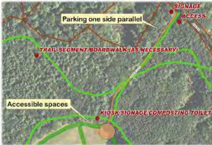
Figure 7 This detail from the Master Plan in the Appendix shows how the parking will be along the existing roadway into the site, with a turnaround (circle) near the cap. This provides non-intrusive parking and access to the cap for people of all abilities.
