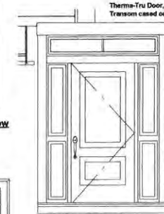
Unit 8 & 9 Entry Door Scale: 1" = 1'-0"
