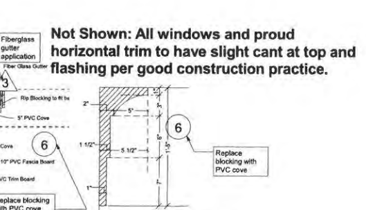
M:3.1 Enlarged Profile of Trim @ Main Eave Scale: 2" = 1'-0"
