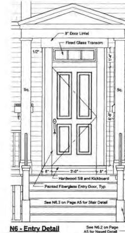
N6 - Entry Detail Scale: 1/2" = 1'-0"
