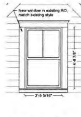
Window Detail Scale: 1/2" = 1'-0"
