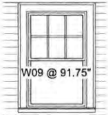
Window Detail Double Hung Scale: 1" = 1'-0"
