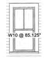
Window Detail Double Hung Scale: 1" = 1'-0"
