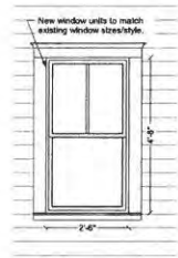
Window Detail Scale: 1/2" = 1'-0"
