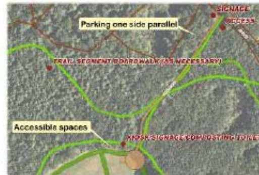
Figure 6 This detail from the Master Plan in the Appendix shows how the parking will be along the existing roadway into the site, with a turnaround (circle) near the cap. This provides non-intrusive parking and access to the cap for people of all abilities.
