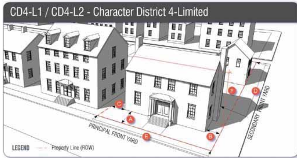
FIGURE 10.5A41.10A DEVELOPMENT STANDARDS CHARACTER DISTRICT 4—LIMITED (CD4-L1/CD4-L2)
