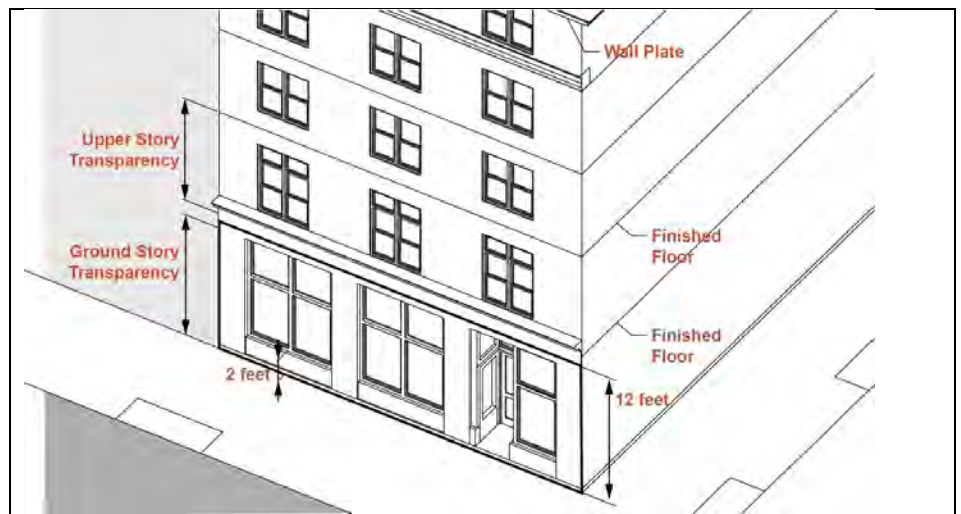
Figure 10.5B25.10 - Ground Floor and Upper Floor Façade Glazing
