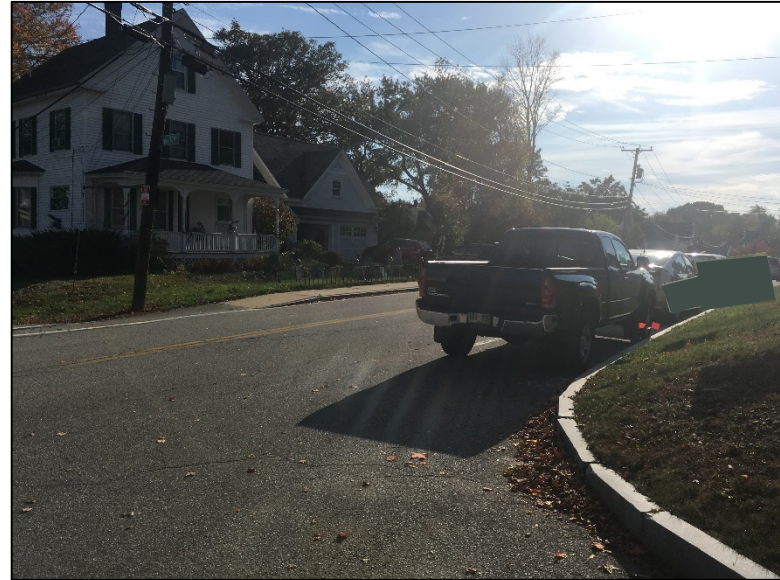
Photo 6: Pedestrian Site Line at Intersection Obstructed by Vehicles
