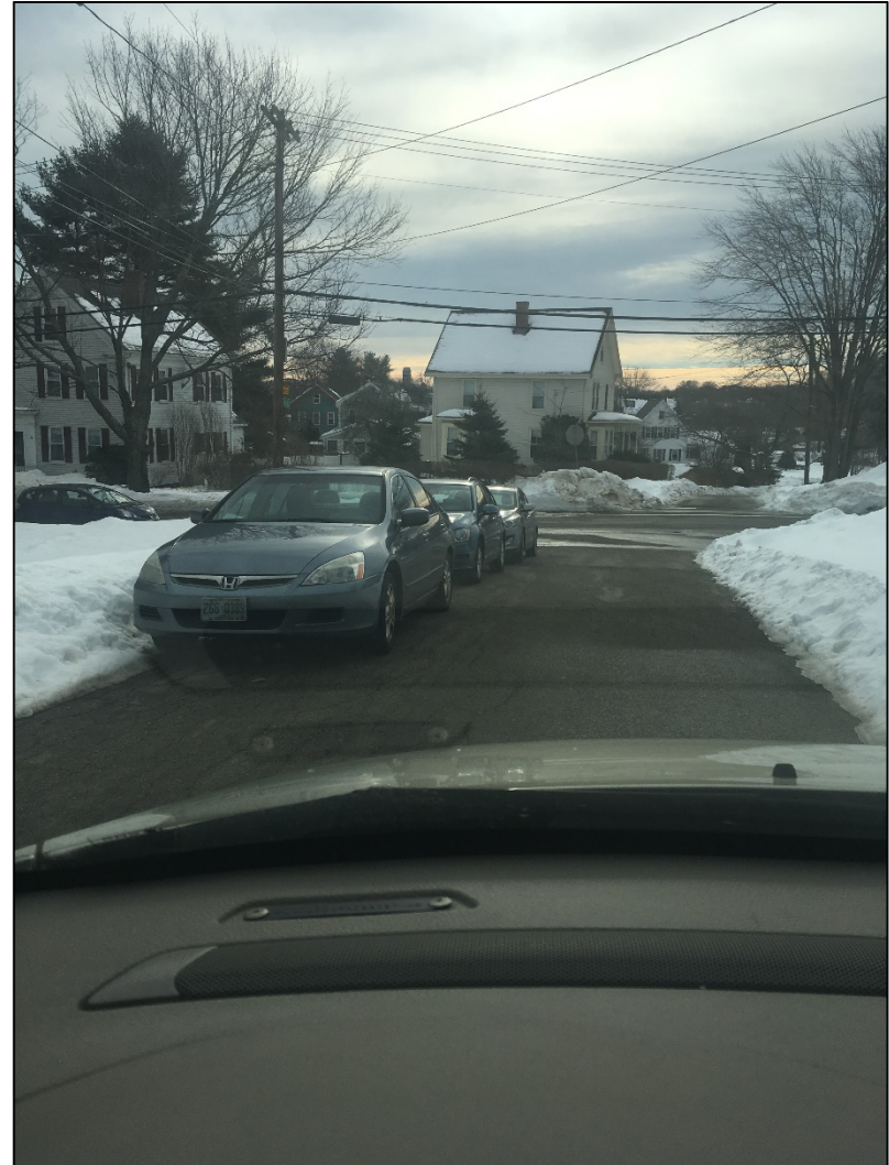
Photo 13: Vehicles along Hunter's Hill (Reduced Street Width Difficult for Standard Vehicles. Likely Inadequate for Emergency Response Vehicles)
