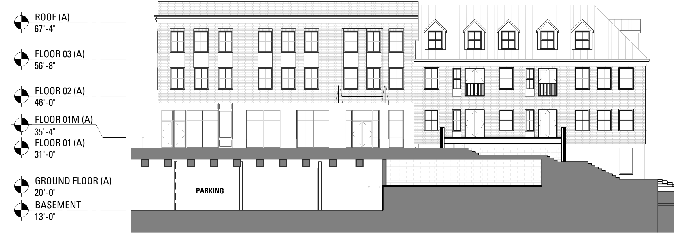
5 BUILDING B - EAST ELEVATION SCALE: 1/16" = 1'-0"
