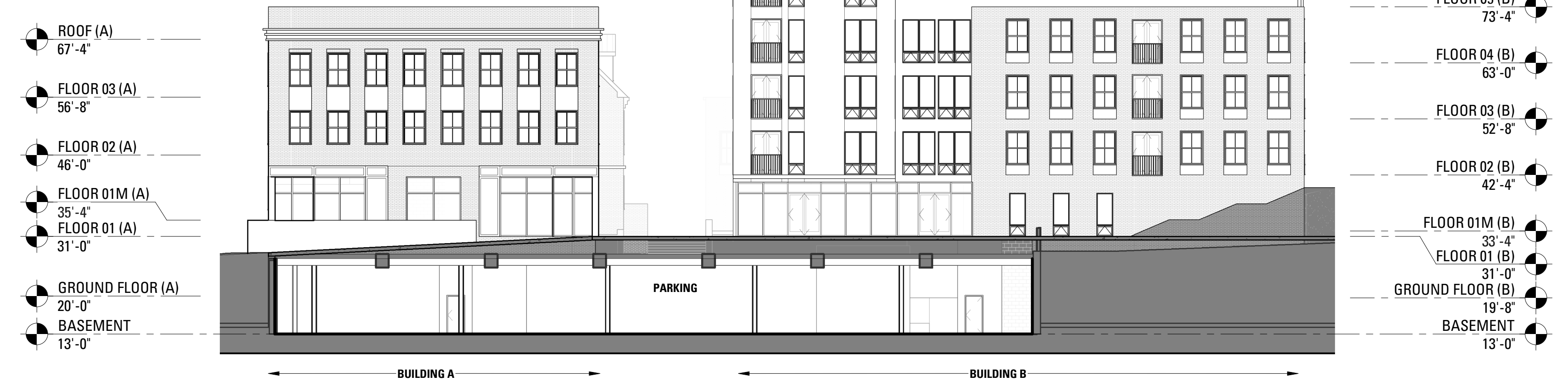
2 SOUTH (LINDEN WAY) ELEVATION SCALE: 1/16" = 1'-0"
