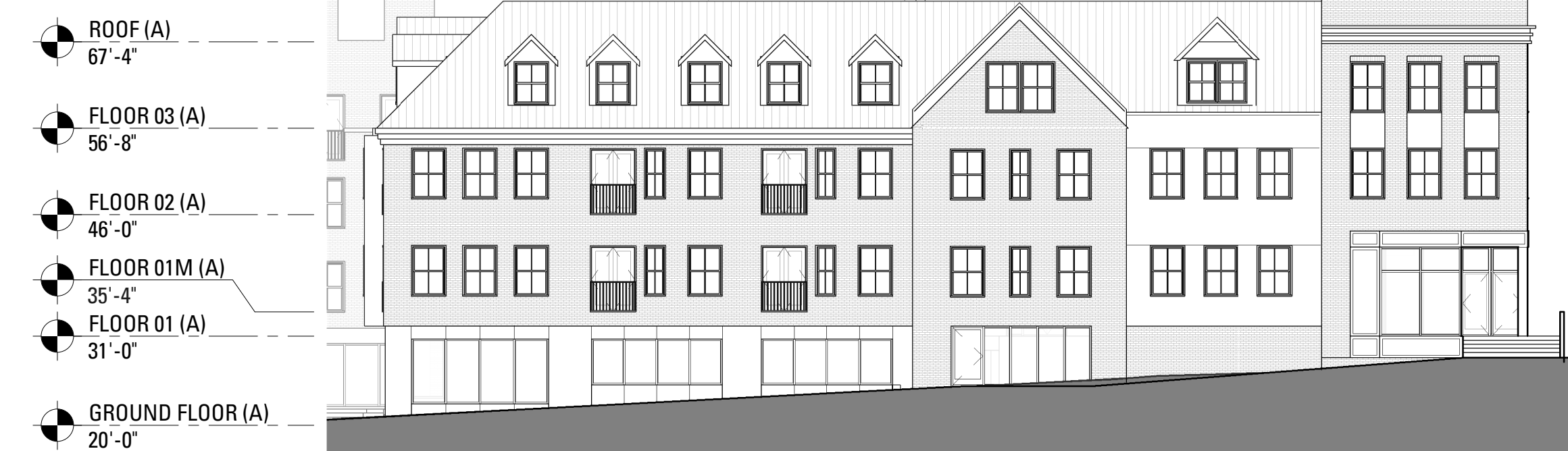
3 BUILDING A - WEST (PENHALLOW STREET) ELEVATION SCALE: 1/16" = 1'-0"
