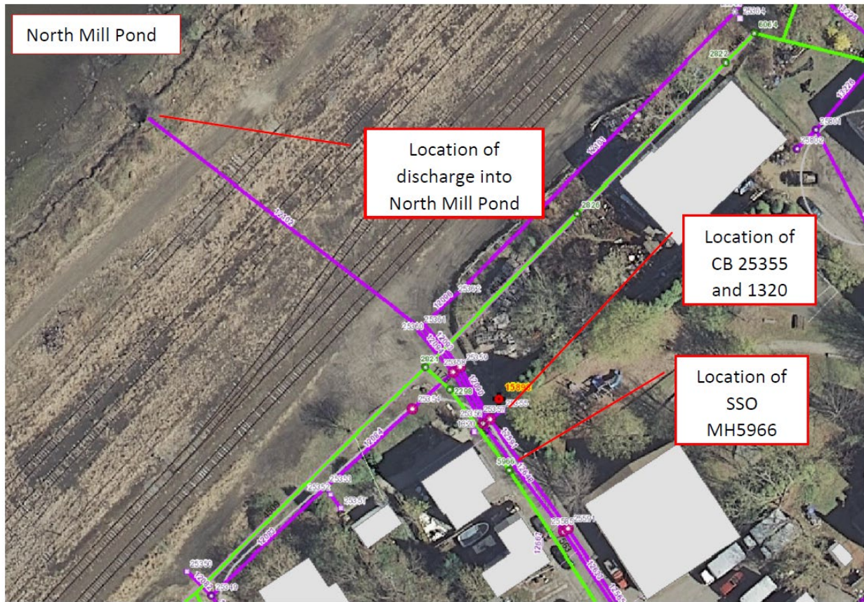
Site Map: Manholes 5966 and 5966a surcharged into catch basins 25355 and 1320, discharging into North Mill Pond
