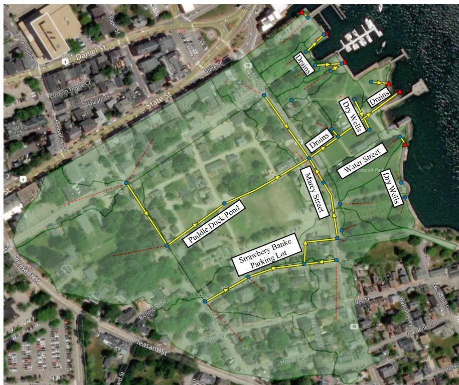
Figure 1: Schematic of Existing Stormwater Infrastructure in and Upgradient of Prescott Park
