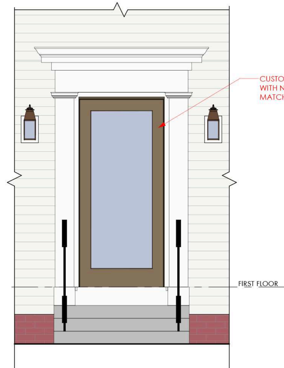
PROPOSED STORM DOOR AT ENTRY (1) 1/2" = 1'-0"
