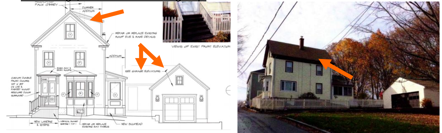
Proposed Alterations and Existing Conditions
