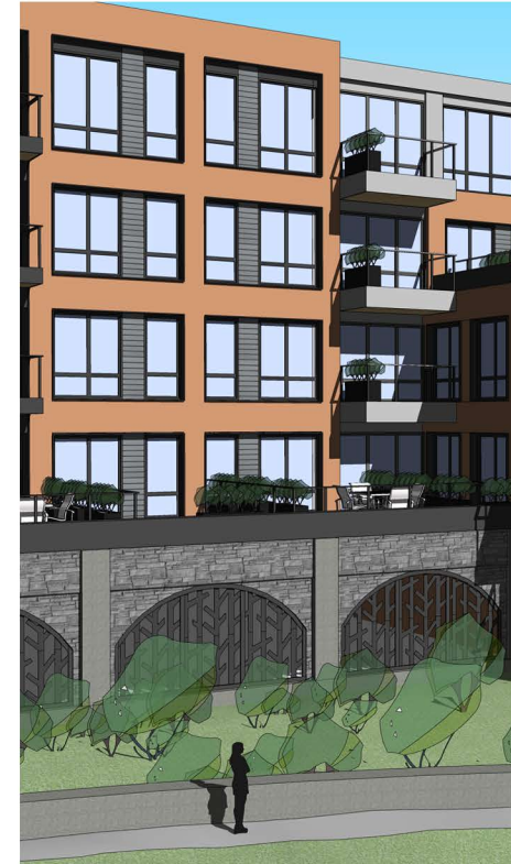
PROJECTING BALCONIES ABOVE. SOLID TEXTURED BASE ELEMENTS WITH HORIZONTAL AND VERTICAL BANDING.
