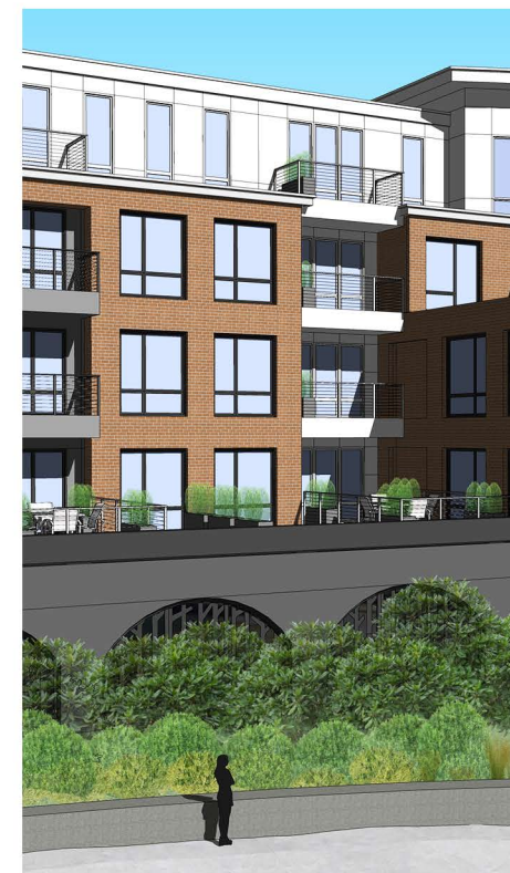
RECESSED BALCONY RIBBONS EXTEND DOWN TO REST ON A SOLID ARCHED BASE ELEMENT THAT CARRIES THE CURVILINEAR THEME TO THE GROUND. DECORATIVE GRILLWORK PROVIDES A BACKDROP FOR THE LANDSCAPED EARTH BERM AND LOW SEATING WALL.
