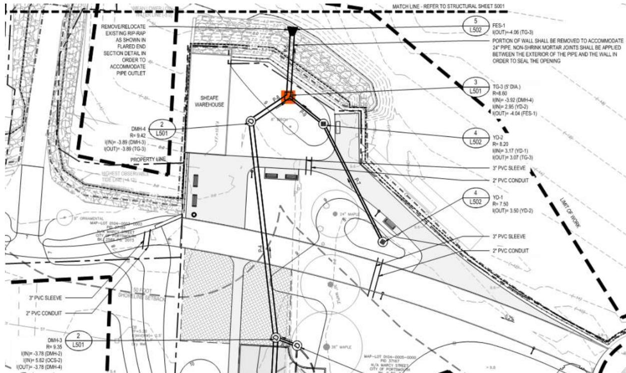
Figure 8: Proposed Tide Gate From Plan Sheet L141
