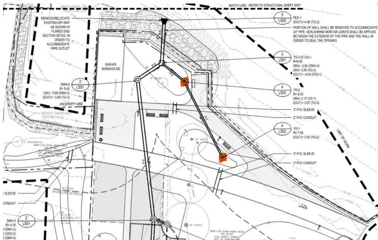
Figure 7: Proposed Catch Basins from Plan Sheet L141
