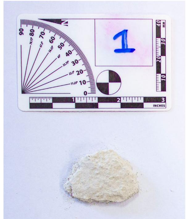
Photograph of the bulk sample before digestion (fluorescent light, color corrected).
