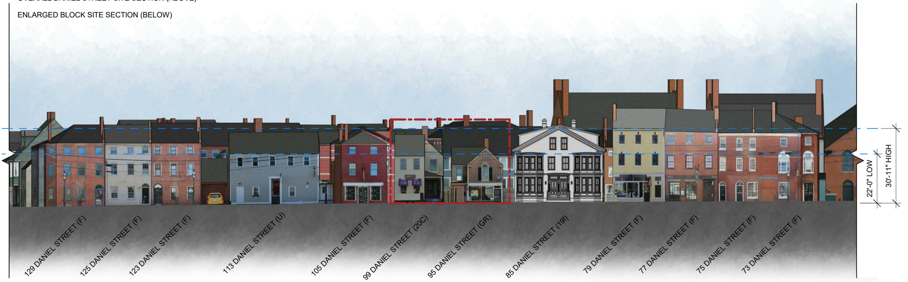
NOTE: ALL DIMENSIONS ON SHEET DEPICT BUILDING EAVE HEIGHT FROM AN ASSUMED AVERAGE GRADE TO UNDERSIDE OF EAVE, ALL DIMENSIONS ARE +/-
