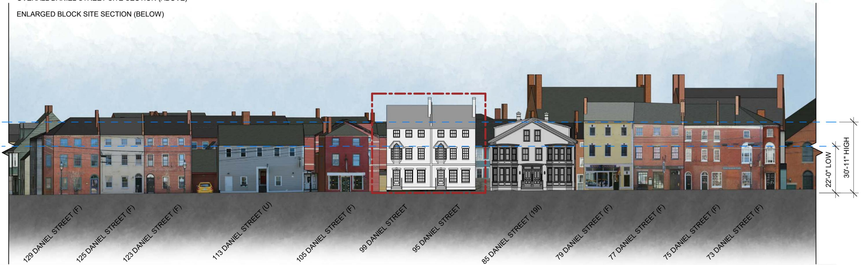
NOTE: ALL DIMENSIONS ON SHEET DEPICT BUILDING EAVE HEIGHT FROM AN ASSUMED AVERAGE GRADE TO UNDERSIDE OF EAVE, ALL DIMENSIONS ARE +/-
