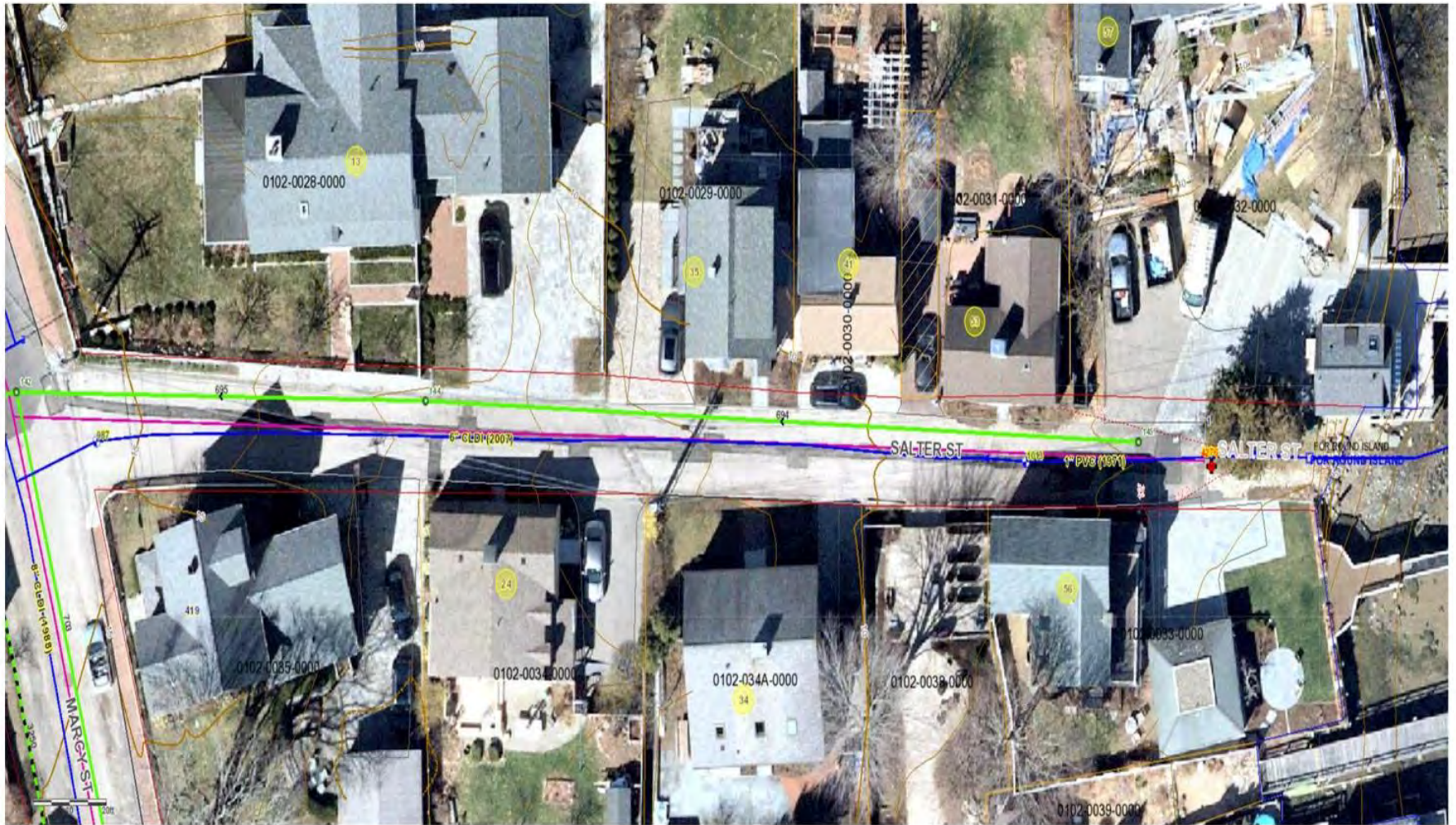
City of Portsmouth Municipal Water (blue), Sewer (green), and Drain (purple) utilities on Salter Street.
