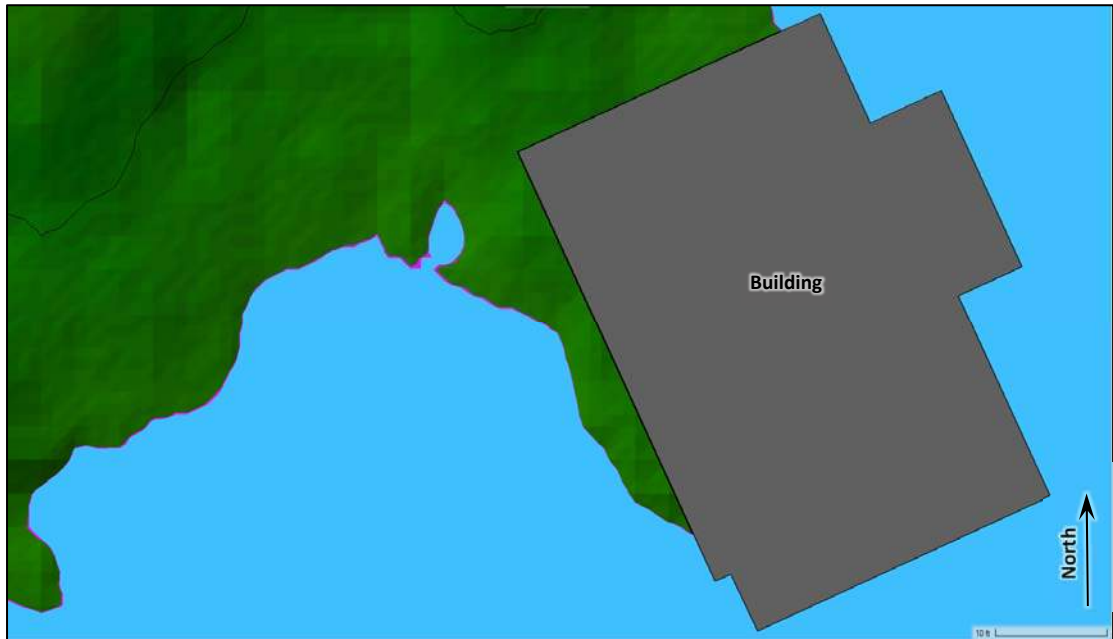
Figure 56 – Detail view of a portion of the shoreline southwest from the bridge showing the inundated areas at the peak water levels calculated with the pre- and post-project 50-year storm models with 1.0 ft SLR. The area shaded blue represents the post-project inundation area. The pink area along the periphery of the blue-shaded area represents the additional area flooded under pre-project conditions.
