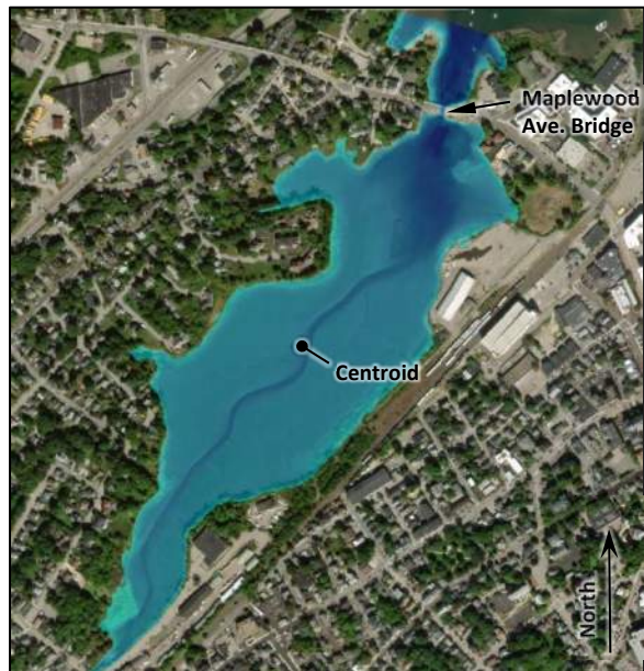
Figure 27 – Inundation area at the MHHW tide stage crest with 1.0 ft SLR for both pre- and post-project conditions
