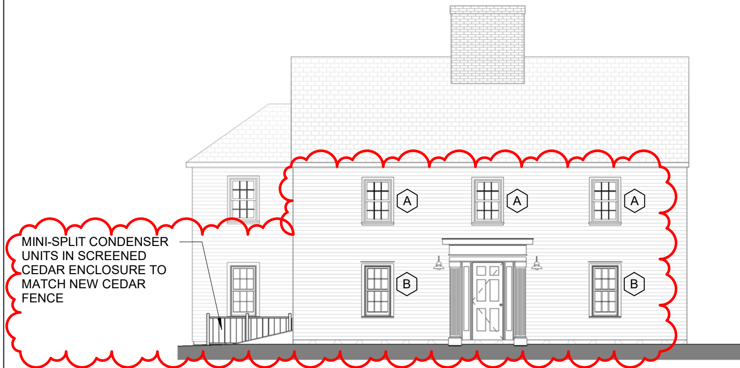
1 NORTH ELEVATION (GATES STREET) - WINDOW TYPE B 1/8" = 1'-0"
