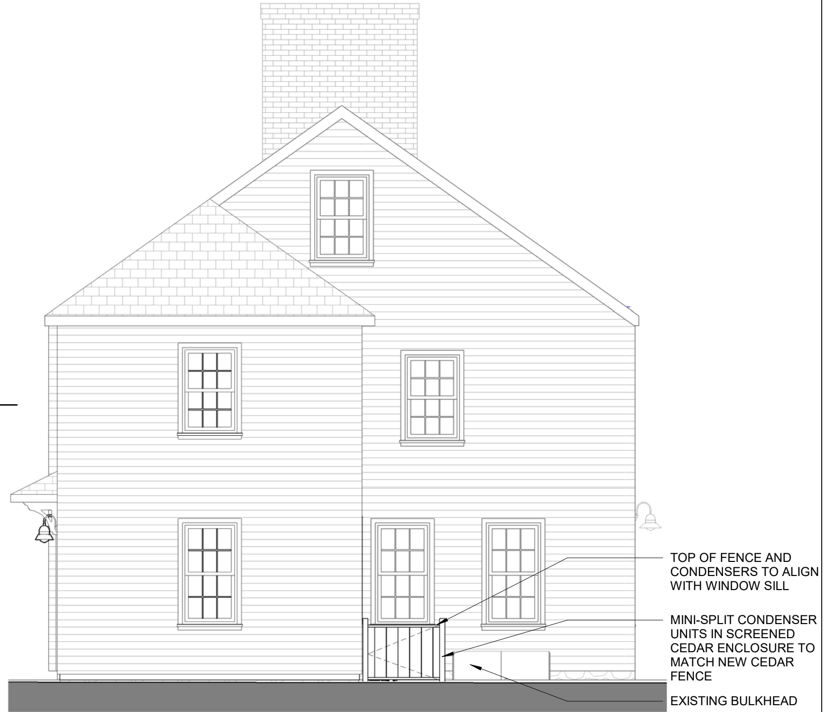
2 EAST ELEVATION (REAR YARD) 1/4" = 1'-0"
