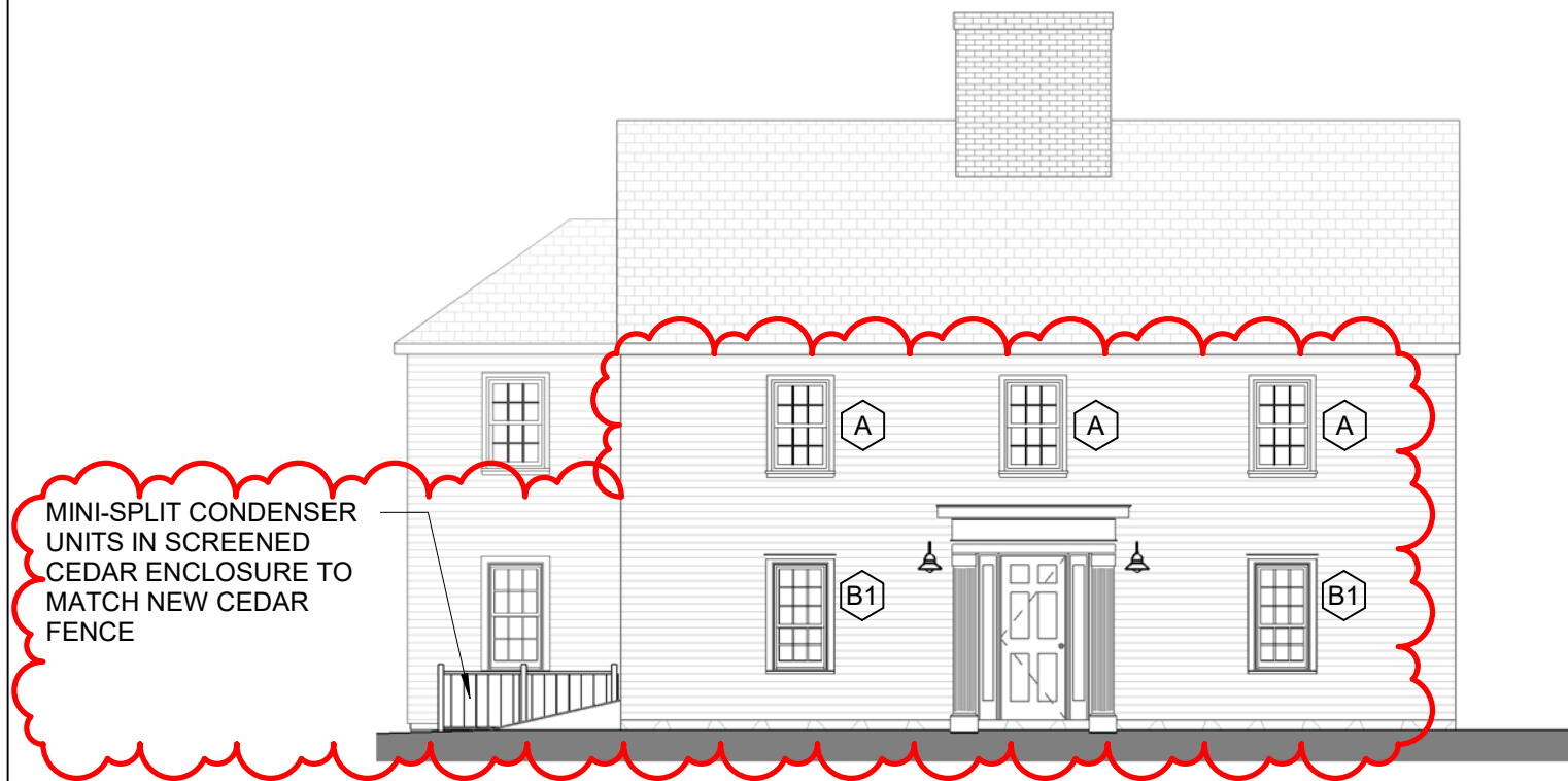
3 NORTH ELEVATION (GATES STREET) - WINDOW TYPE B1 1/8" = 1'-0"
