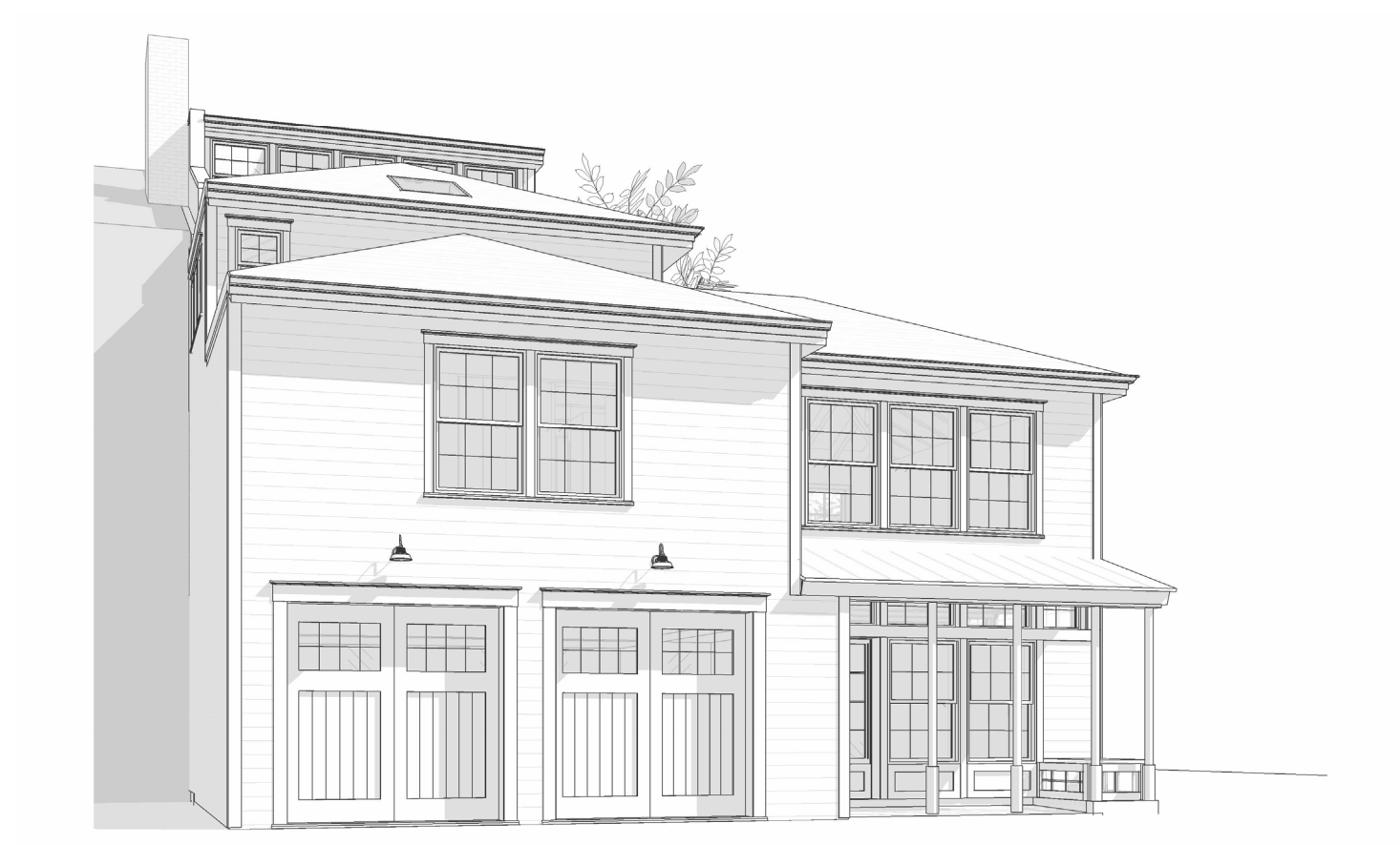
PROPOSED ALTERNATE - NO EAVE OVERHANG
