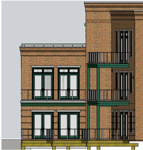
② NE ELEVATION EX. FAILING DOORS (RIVER SIDE) Scale: 3/32" = 1'-0"
