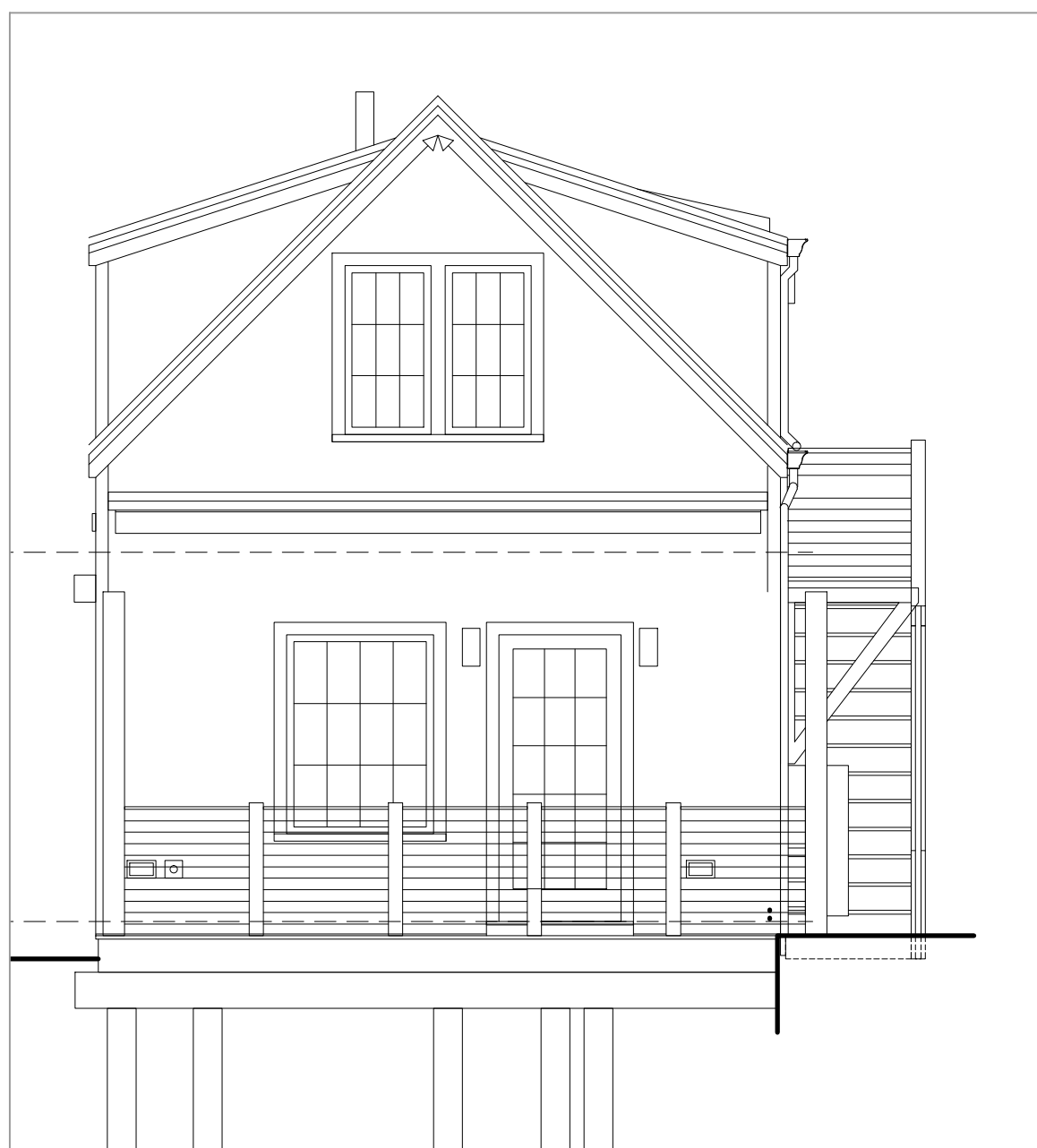
Existing East Elevation
