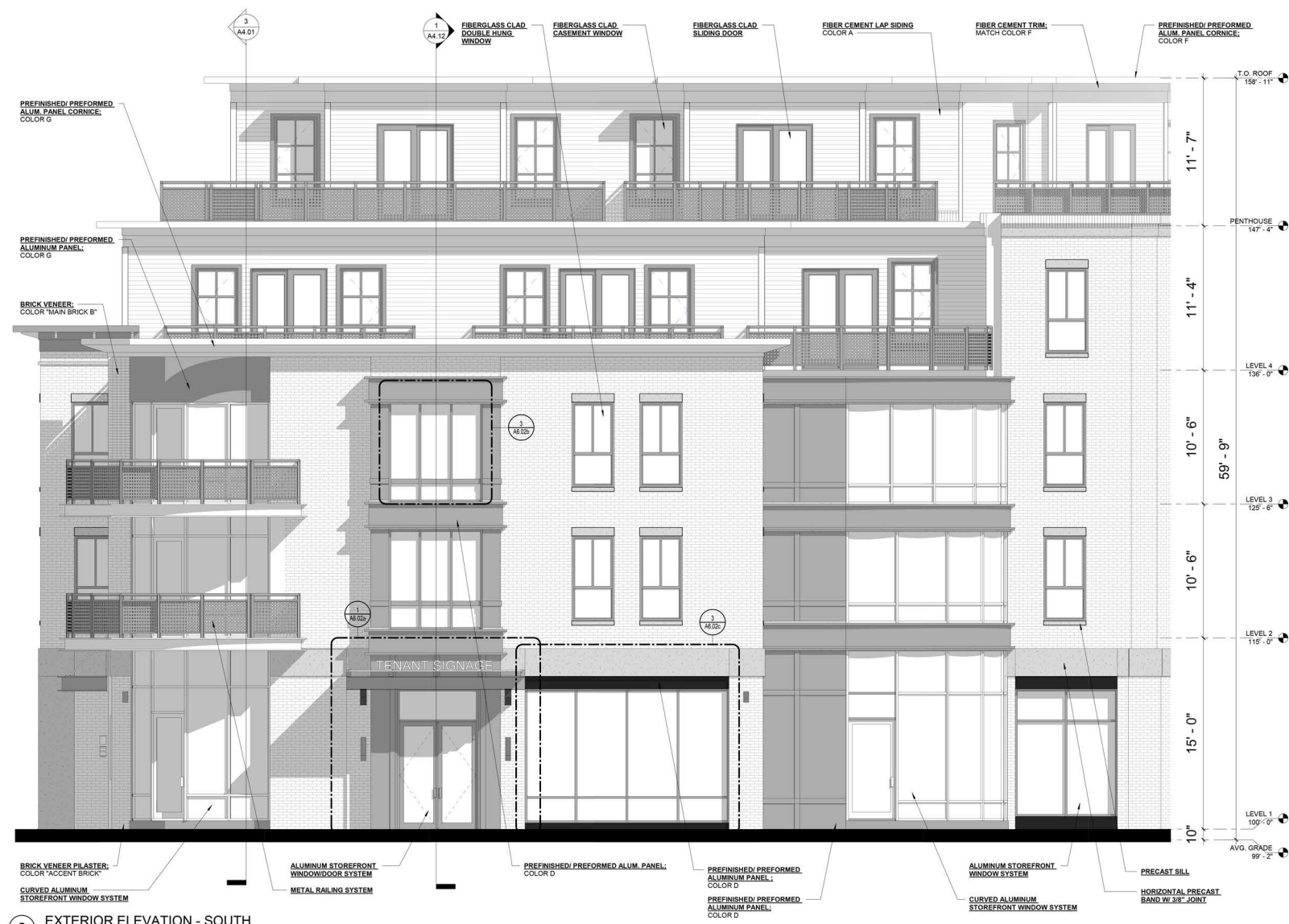
2 EXTERIOR ELEVATION - SOUTH SCALE: 1/4" = 1'-0" REF SHEET: 1 / A1.01
