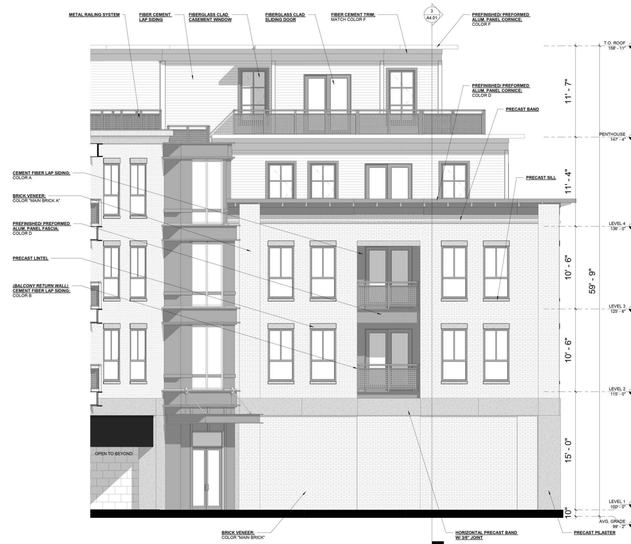
1 EXTERIOR ELEVATION - NORTH SCALE: 1/4" = 1'-0" REF SHEET: 1 / A1.01
