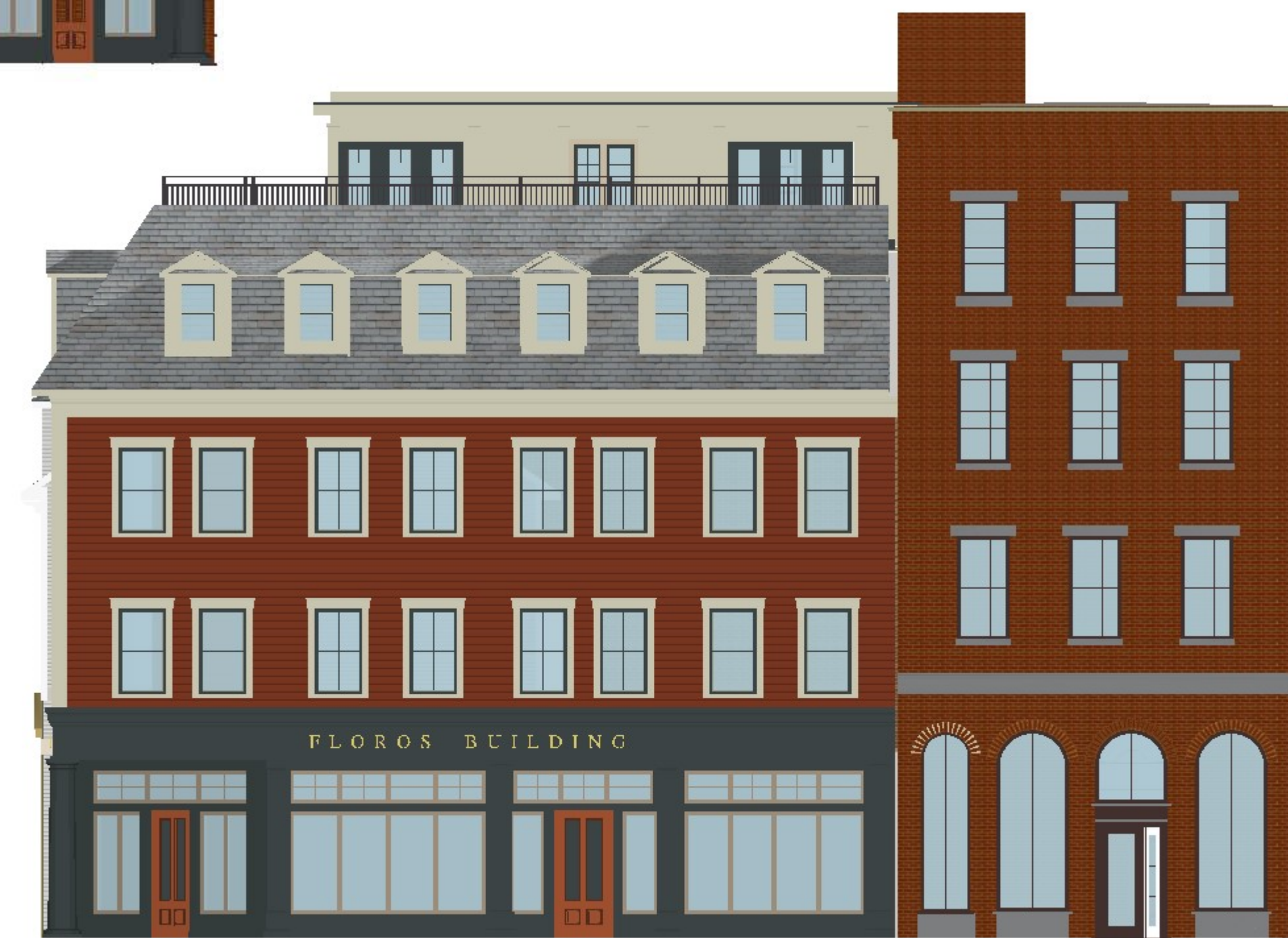
STATE STREET ELEVATION SCALE: 1/8" = 1'-0"
