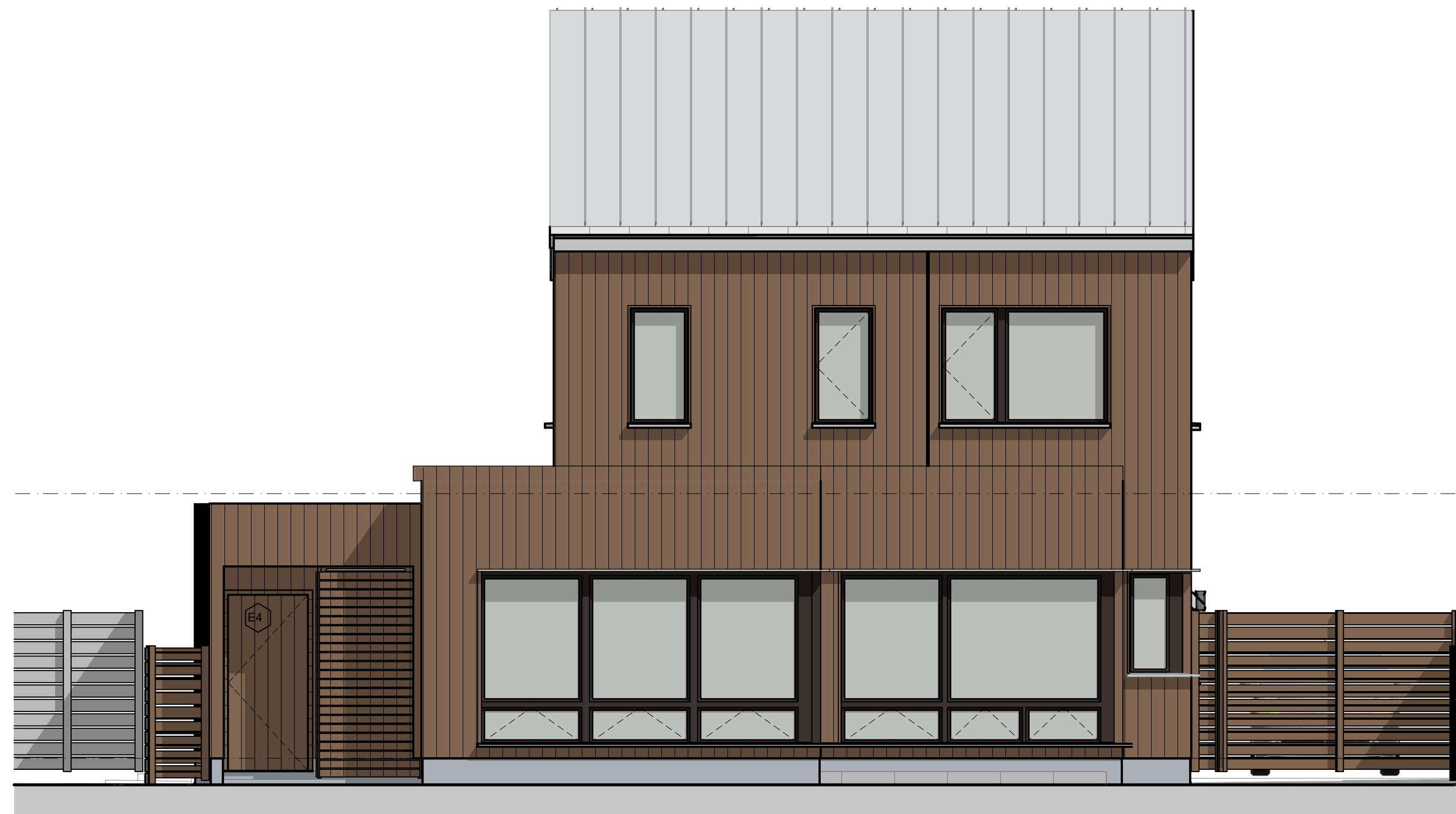
2 EXISTING BACK ELEVATION - SOUTHWEST SCALE: 1/4" = 1'-0"
