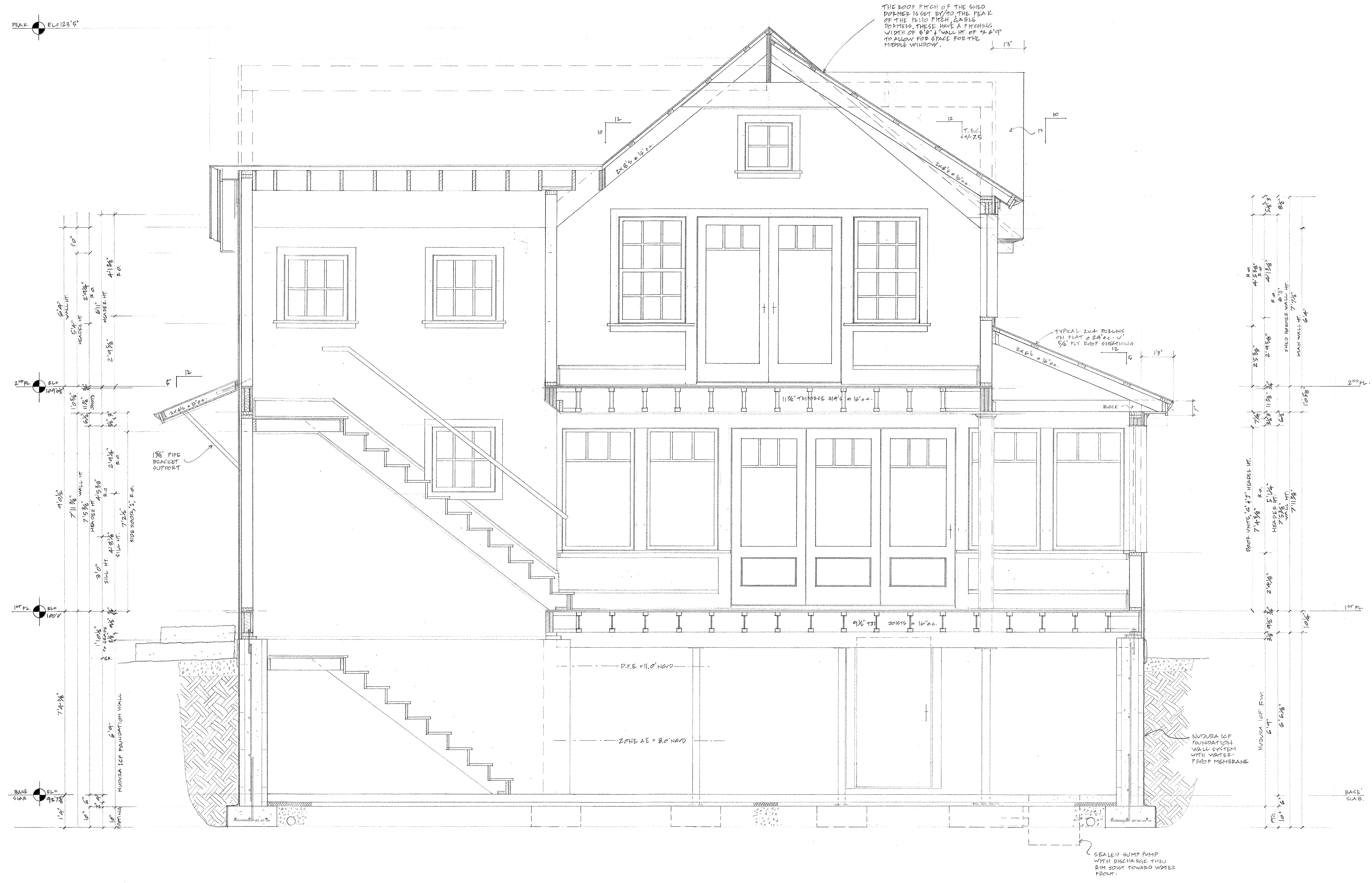
① SECTIONAL VIEW, NORTH/SOUTH (LEFT/RIGHT) 1/2"=1'0"
