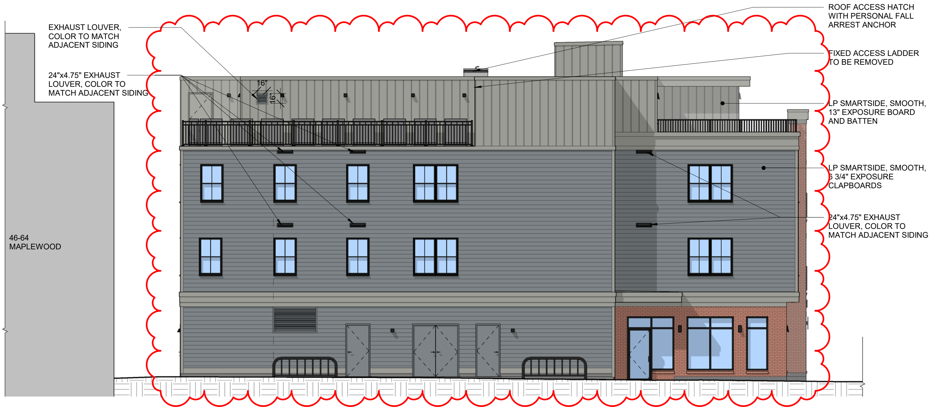
1 EAST ELEVATION (PUBLIC WALKWAY) 1/8" = 1'-0"
