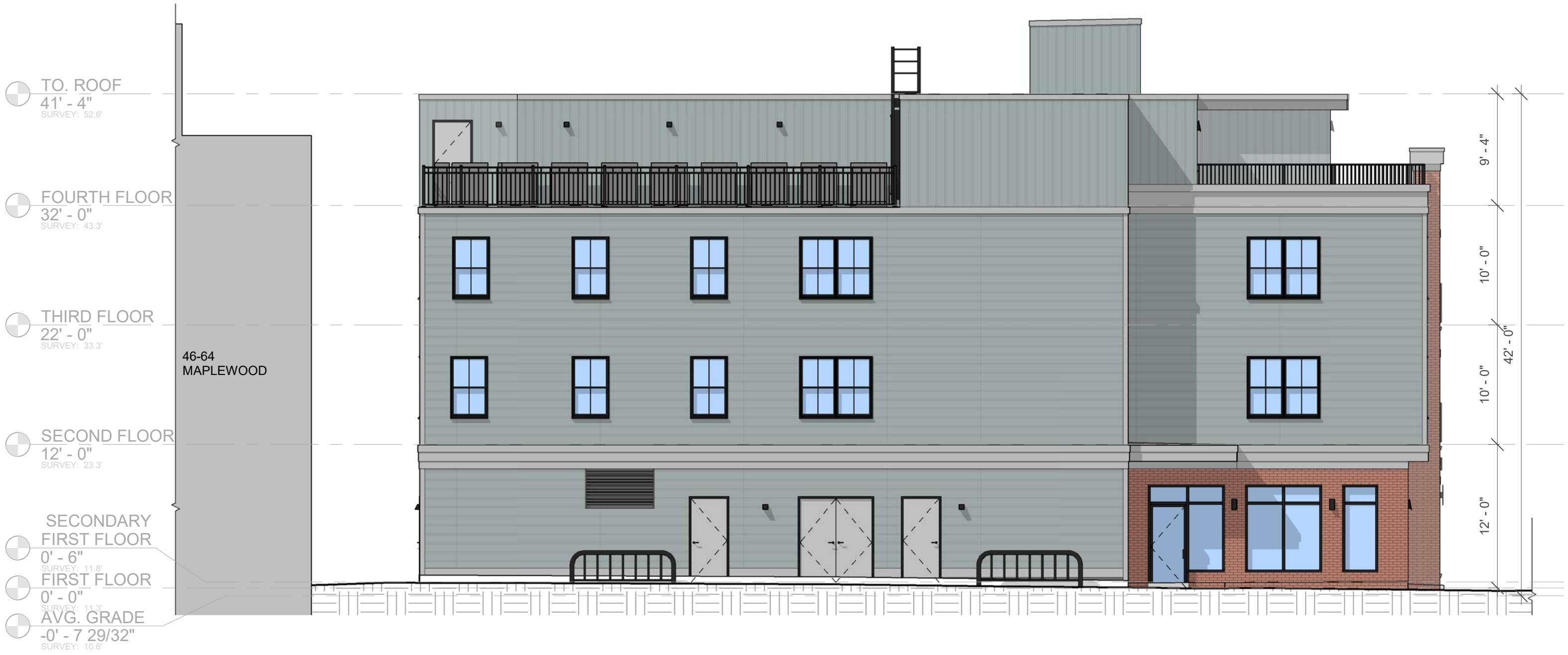
1 EAST ELEVATION (PUBLIC WALKWAY) 1/8" = 1'-0"
