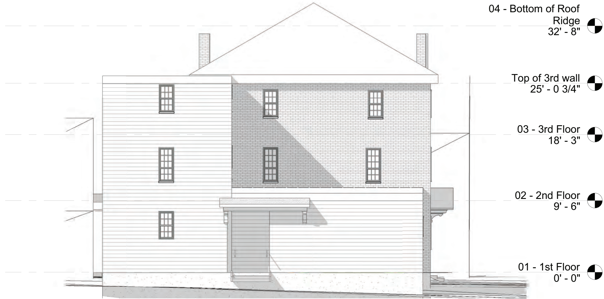
Existing Elevation - South | Scale: 1"=1/8"
