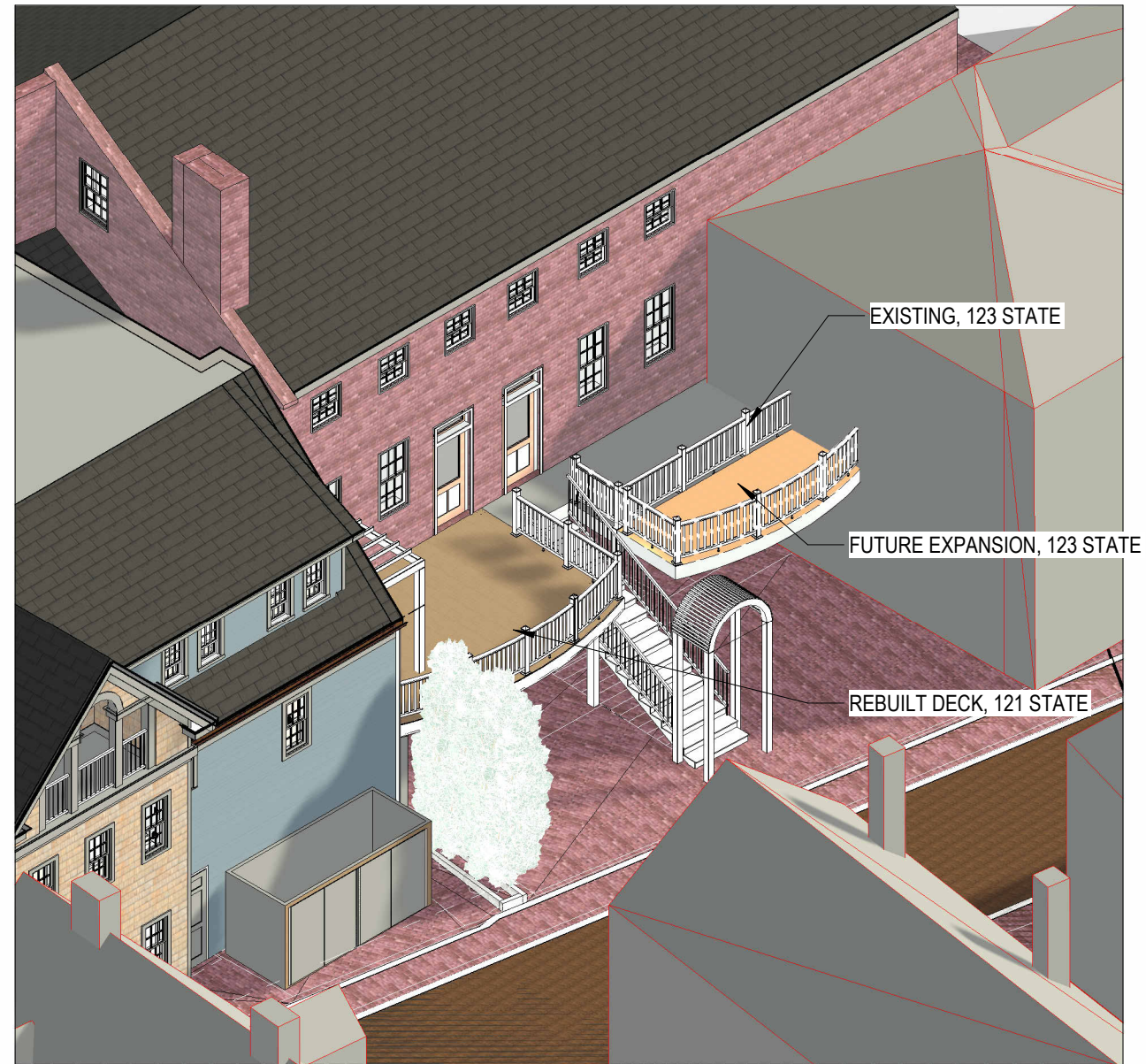
1 AXONOMETRIC, NE PROPOSED
