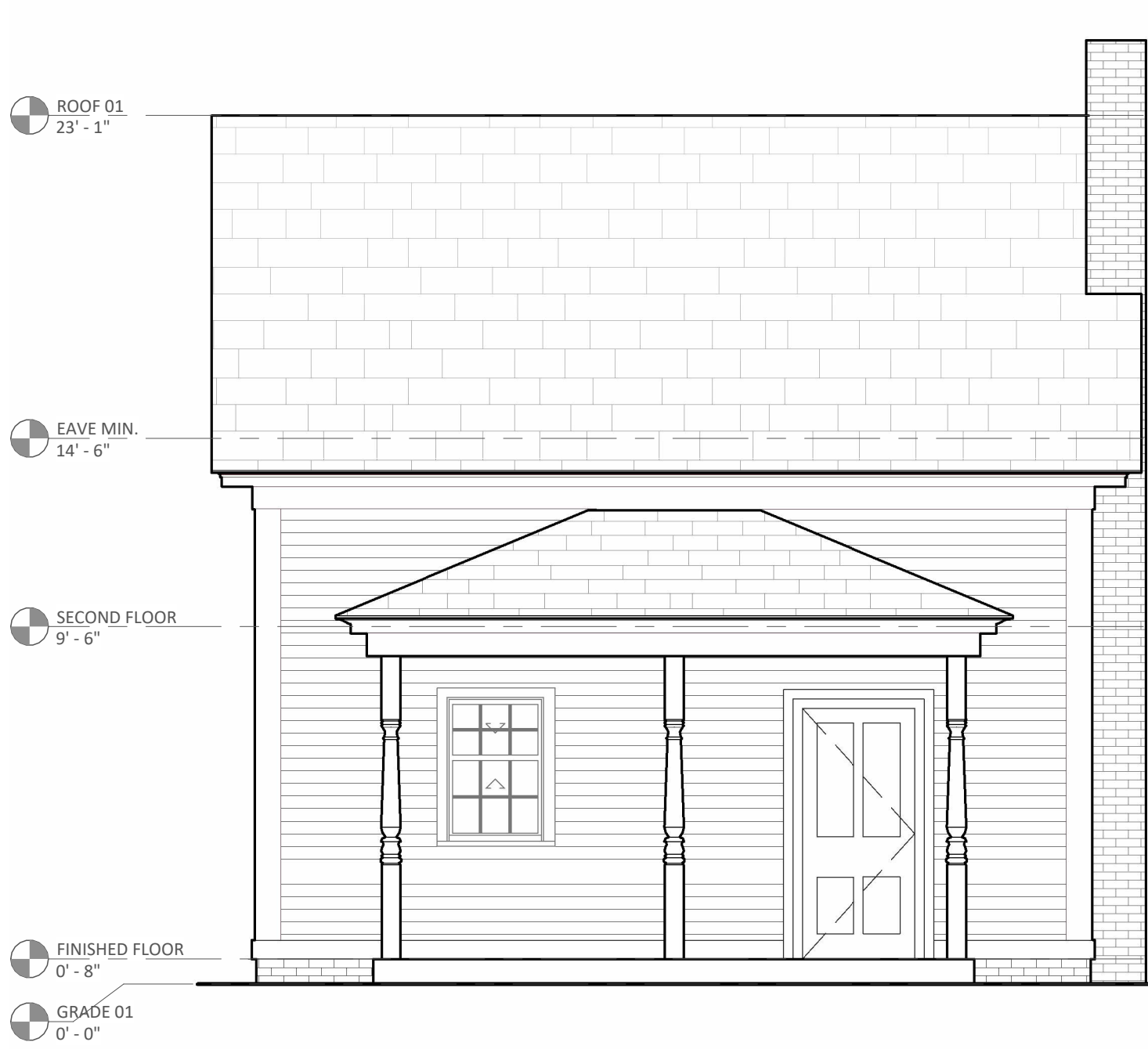
PROPOSED NORTH ELEVATION 1/4" = 1'-0"
