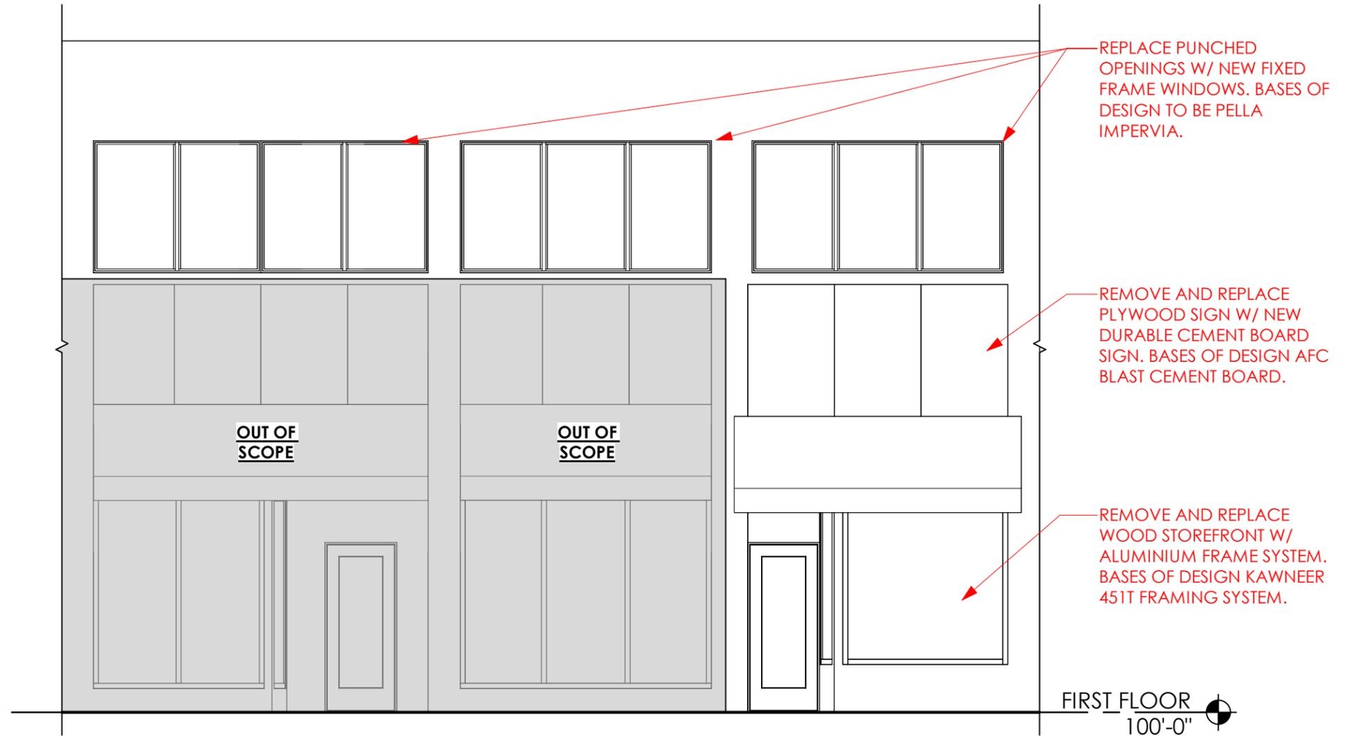
REPLACE PUNCHED OPENINGS W/ NEW FIXED FRAME WINDOWS. BASES OF DESIGN TO BE PELLA IMPERVIA.
