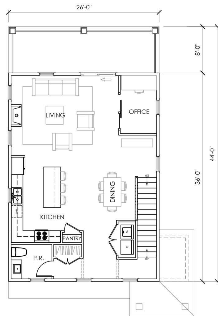
FIRST FLOOR PLAN 1/8" = 1'-0"
