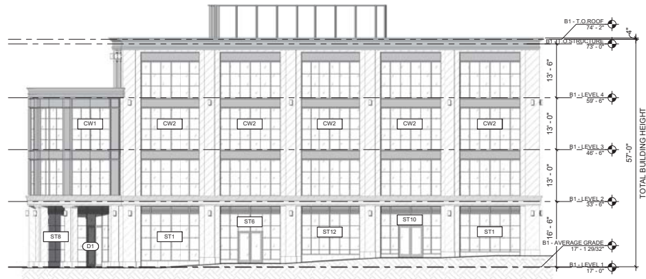
1 B1 - East Elevation 3/32" = 1'-0"
