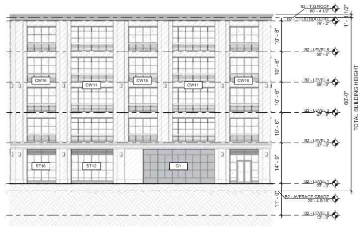
1 B2 - North Elevation 3/32" = 1'-0"
