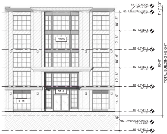
3 B2 - East Elevation 2 3/32" = 1'-0"
