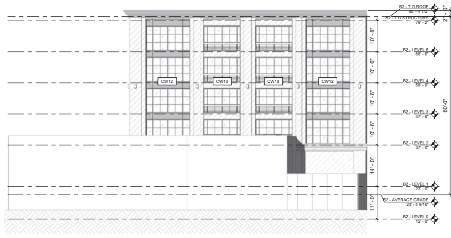
5 B2 - North-West Elevation 3/32" = 1'-0"
