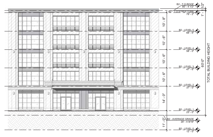
2 B2 - East Elevation 1 3/32" = 1'-0"
