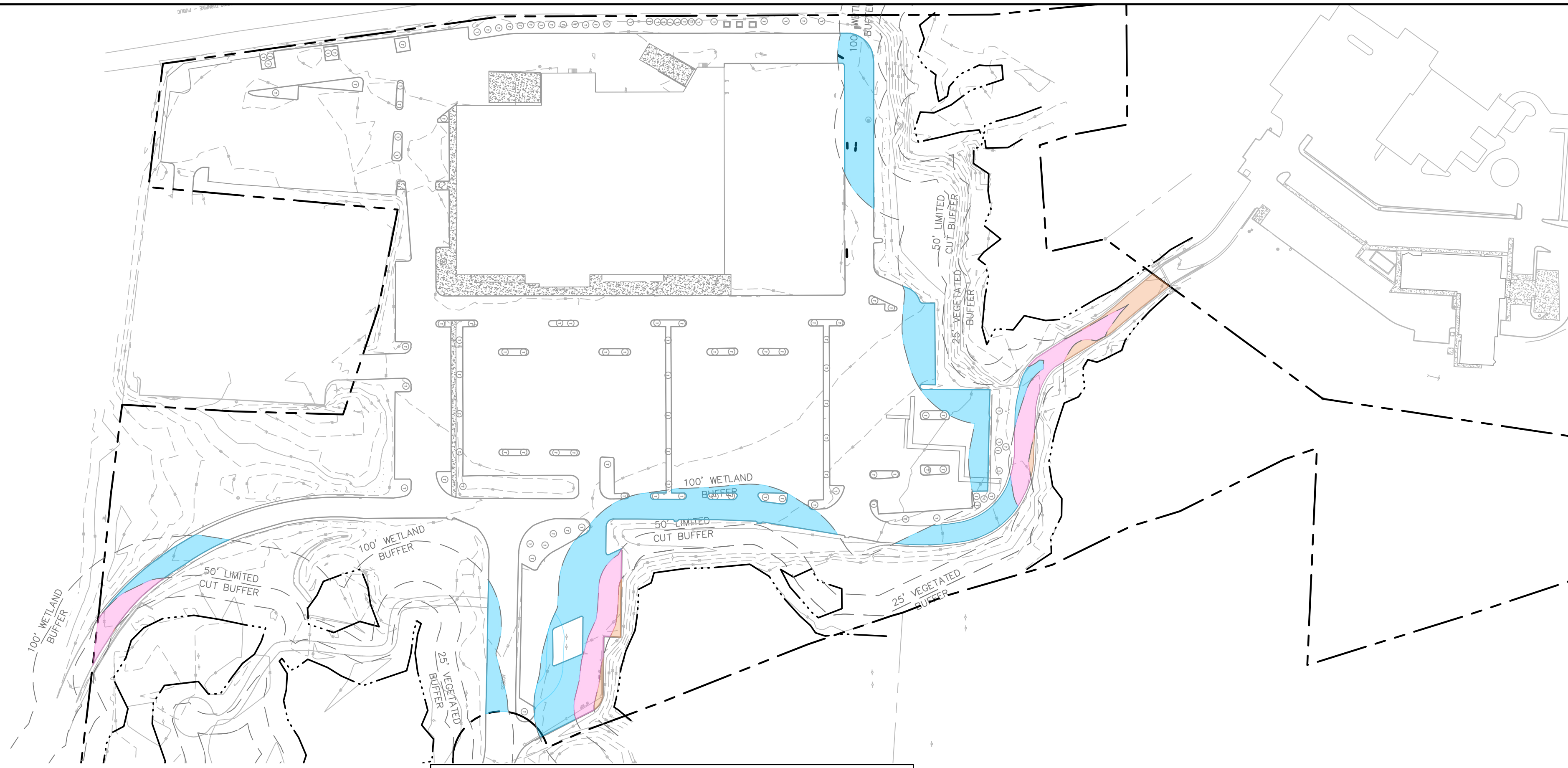
EXISTING WETLAND BUFFER IMPERVIOUS SURFACE SCALE 1" = 100'
