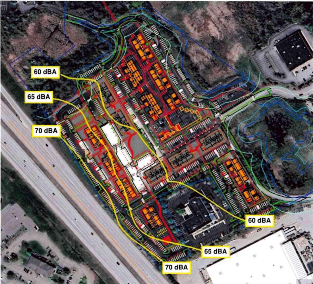
Figure 6. Adjusted 60, 65, and 70 dBA noise contours (5 ft elevation) overlaid upon the Project site diagram based upon Year 2022 traffic data, with mitigation barrier.
