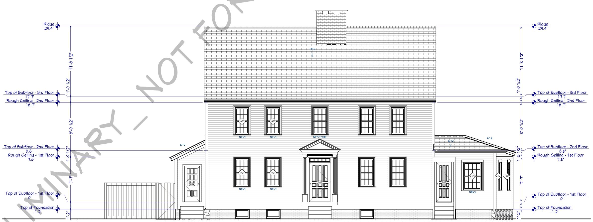
PROPOSED NORTH ELEVATION | FRONT VIEW SCALE: 1/4" = 1'-0"
