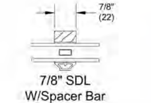
Simulated Divided Lite with Spacer Bar (SDLS)
