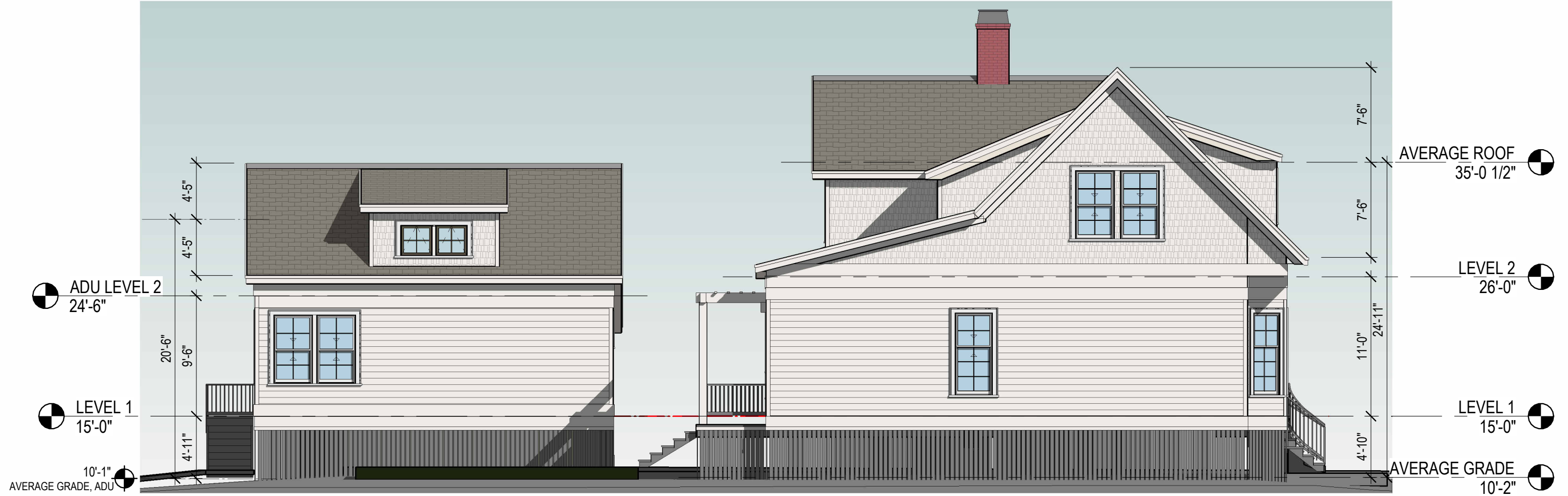
1 EAST ELEVATION (SIDE) 1/8" = 1'-0"
