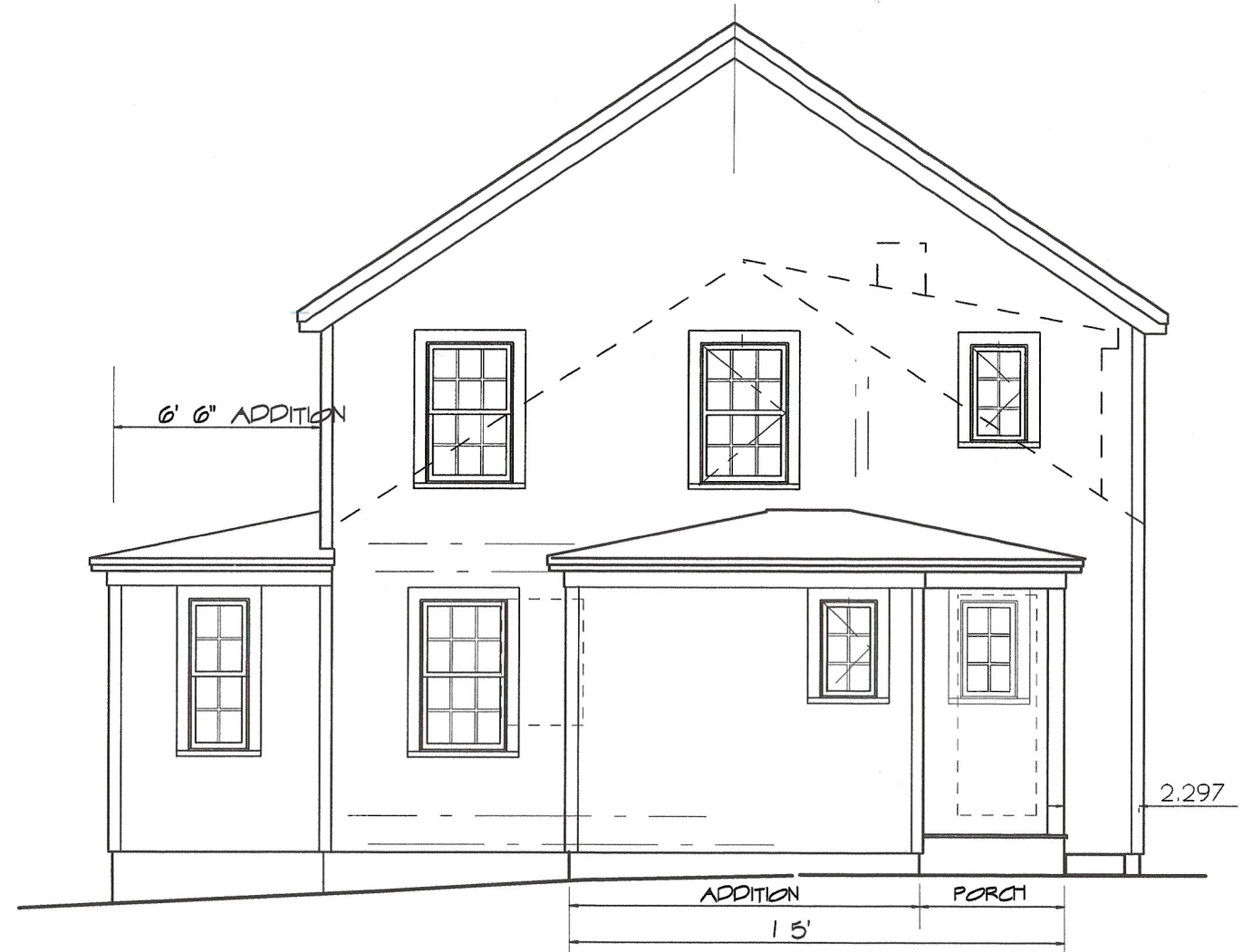
GATES ST ELEVATION SCALE : 3/16" = 1'-0"
