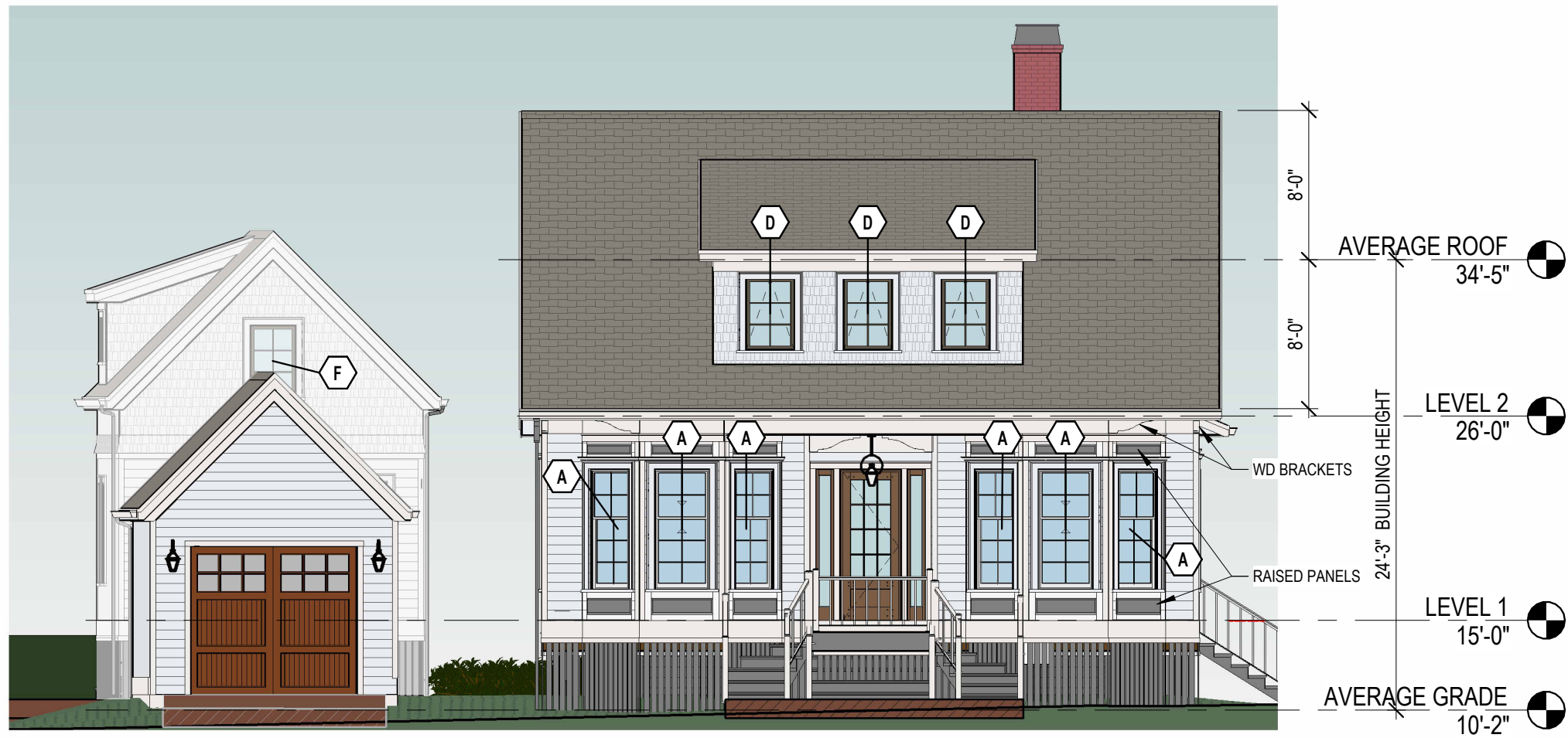
2 NORTH ELEVATION - PRAY ST (FRONT) 1/8" = 1'-0"
