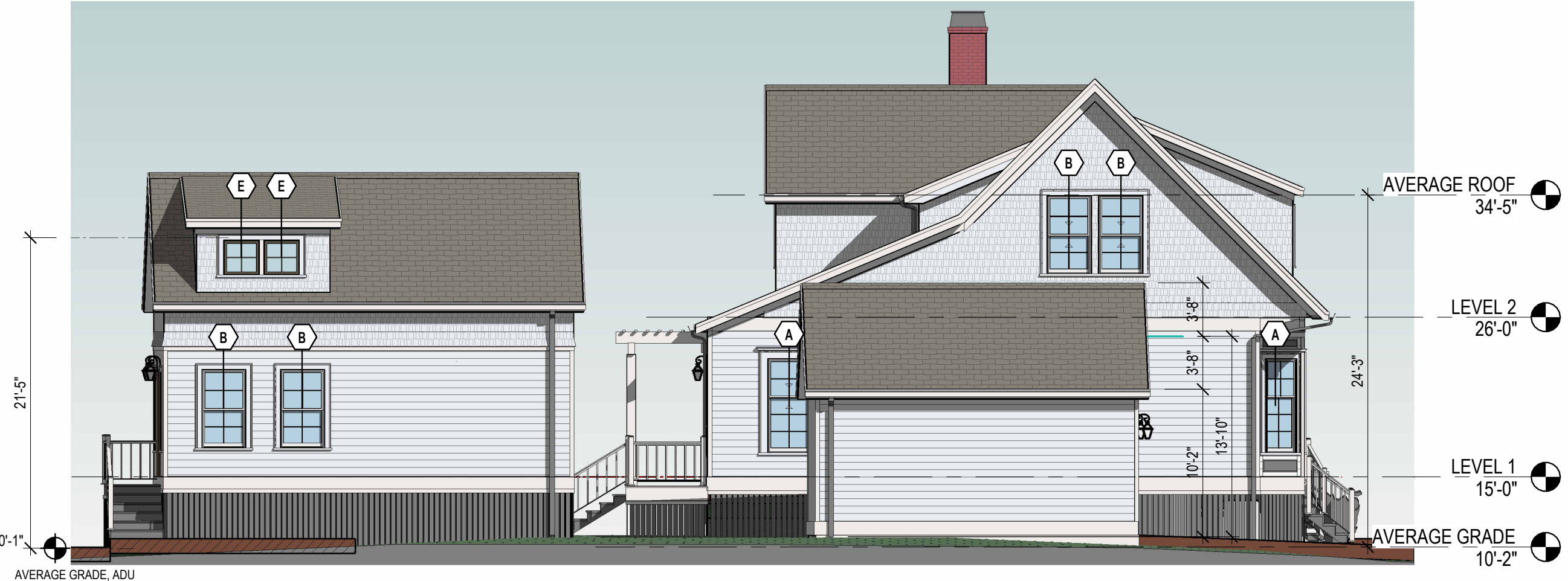
1 EAST ELEVATION (SIDE) 1/8" = 1'-0"
