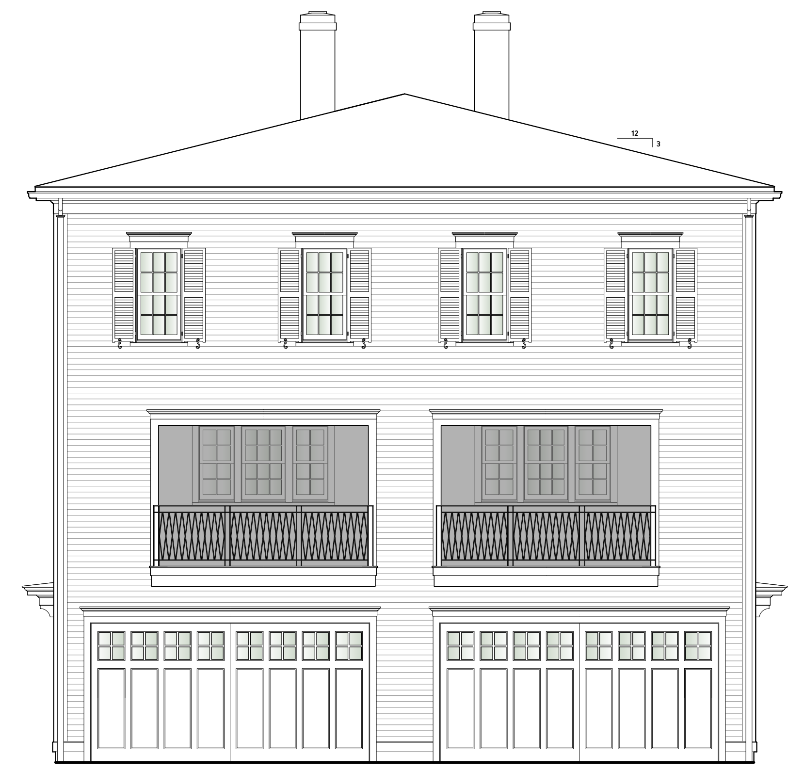
4 BUILDING B: NORTH (REAR) ELEVATION Scale: 3/16" = 1'-0"
