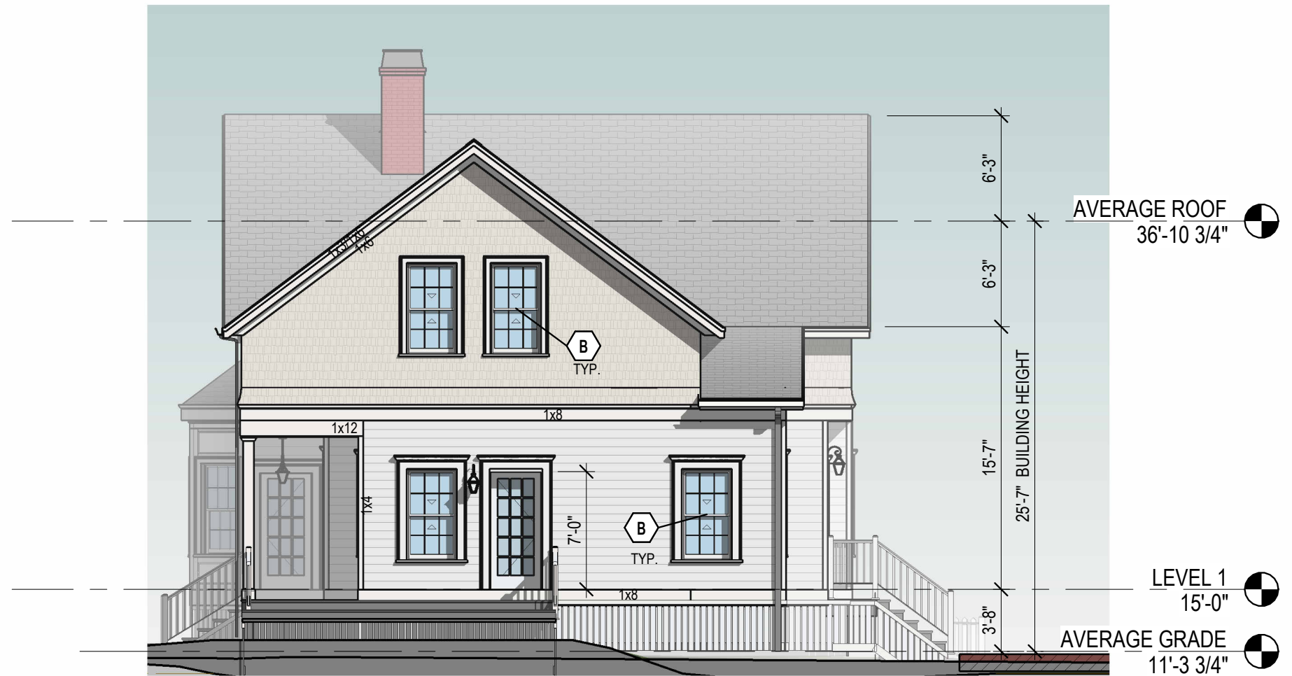
2 SOUTH ELEVATION (SIDE) 1/8" = 1'-0"
