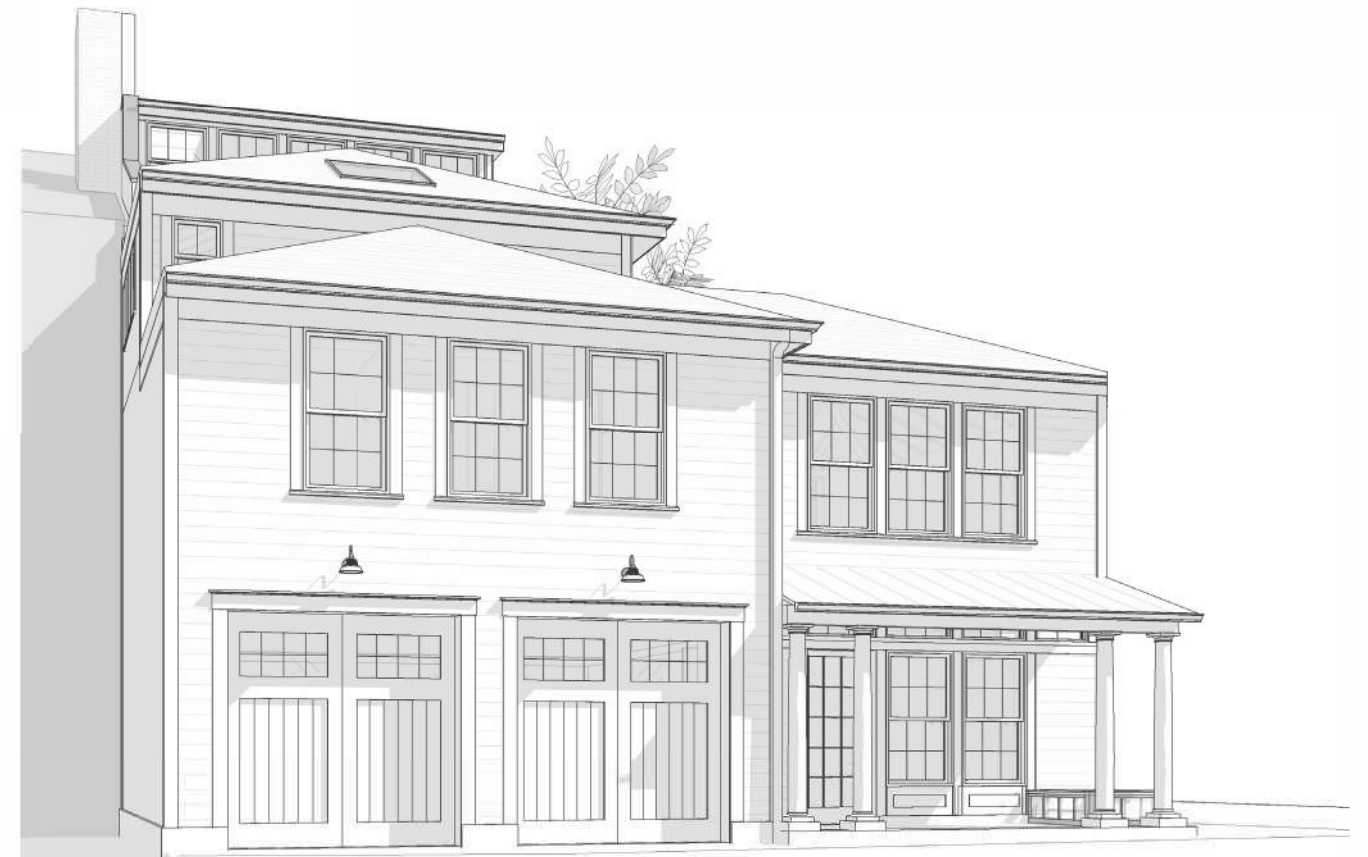
ALTERNATE 2 - NO EAVE OVERHANG (BOTH SIDES)
