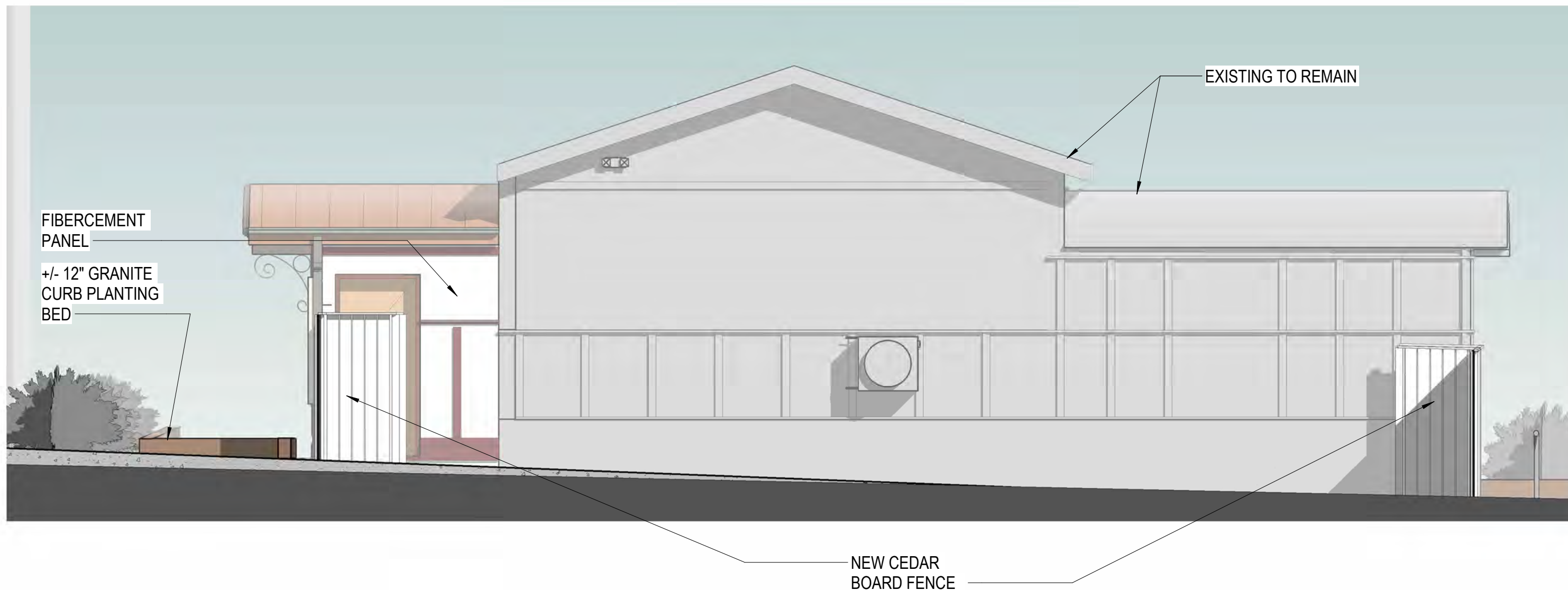
1 GILLEY'S NORTH ELEVATION TRASH ENCLOSURE 1/4" = 1'-0"
