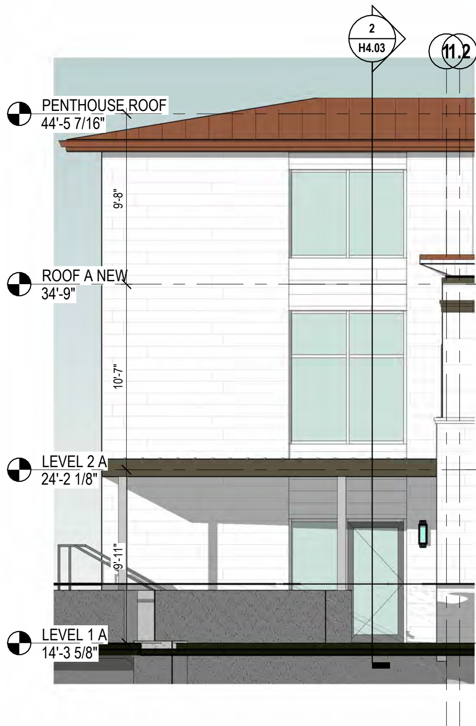
1 ELEVATION - BACK ENTRANCE AND STAIR 3/16" = 1'-0"
