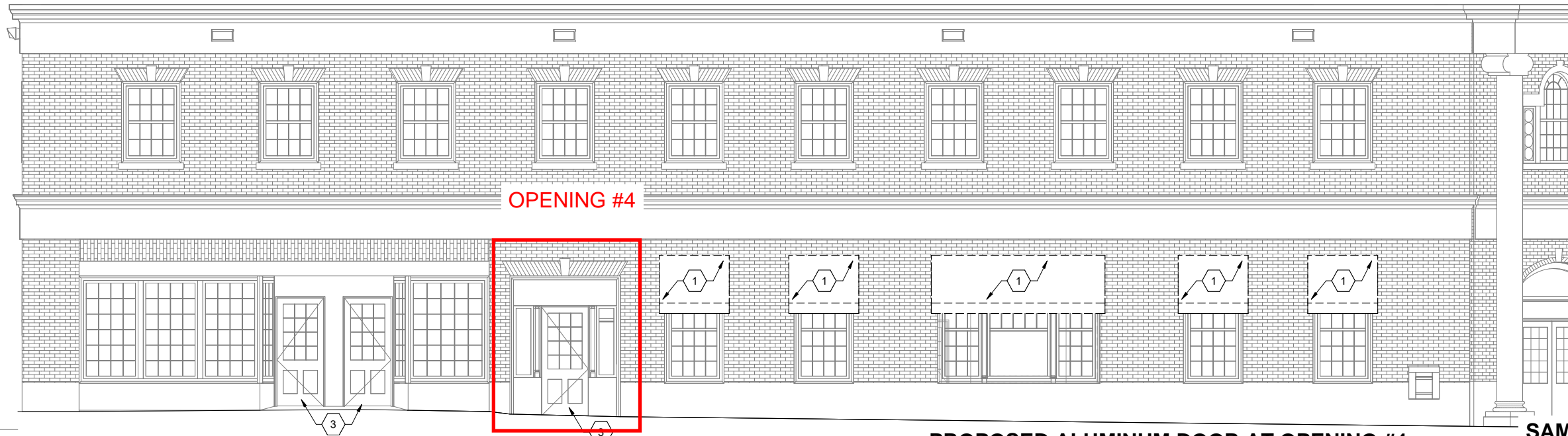
PROPOSED ALUMINUM DOOR AT OPENING #4 DOOR TO BE FACTORY PAINTED TO MATCH EXISTING
