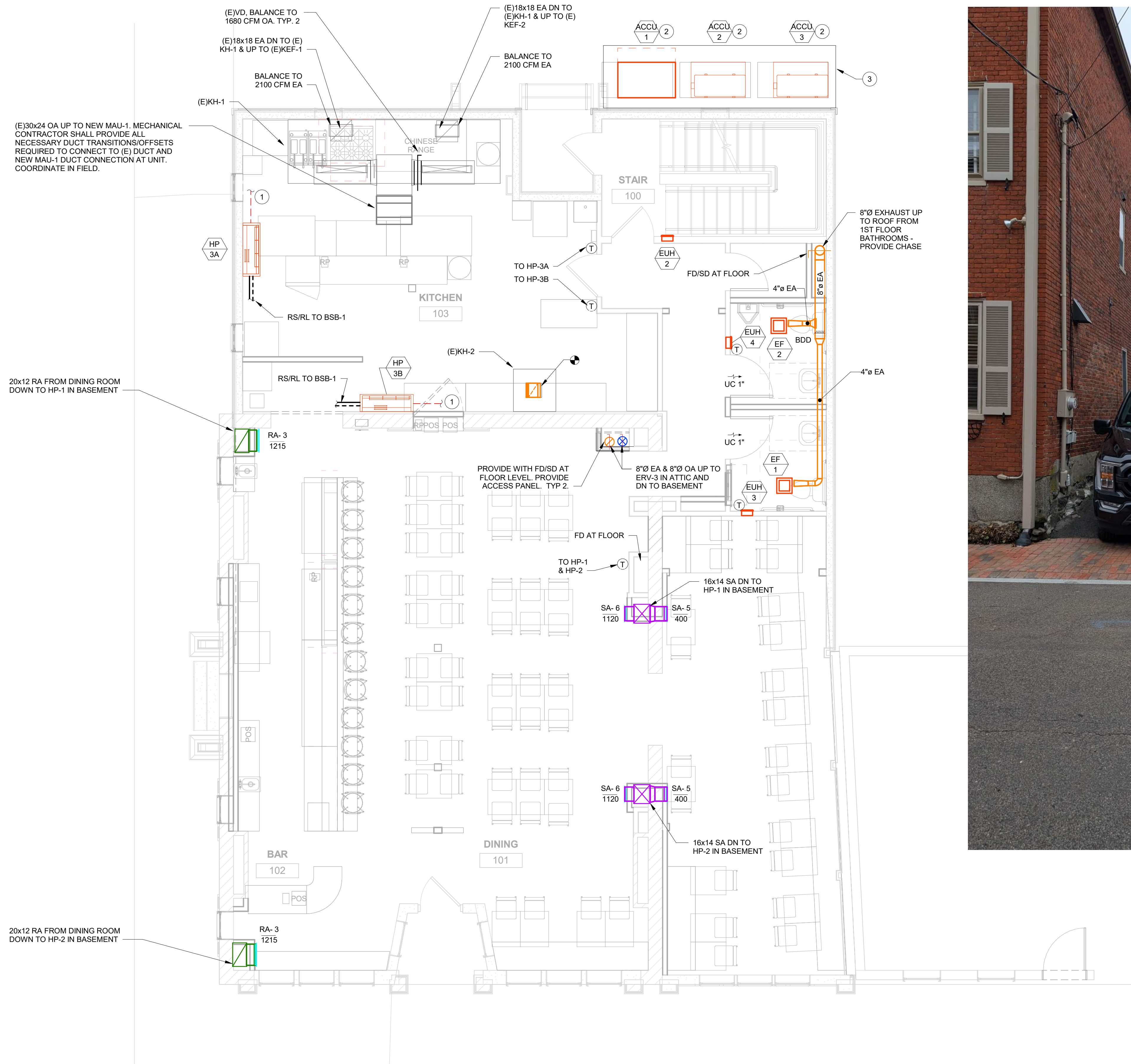
① First Floor Plan - HVAC 1/4" = 1'-0"
