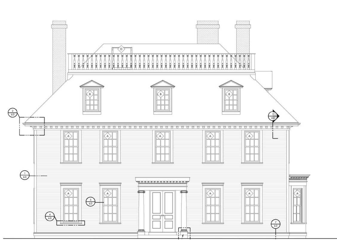
① PREVIOUSLY APPROVED WEST ELEVATION WITHOUT SHUTTERS
