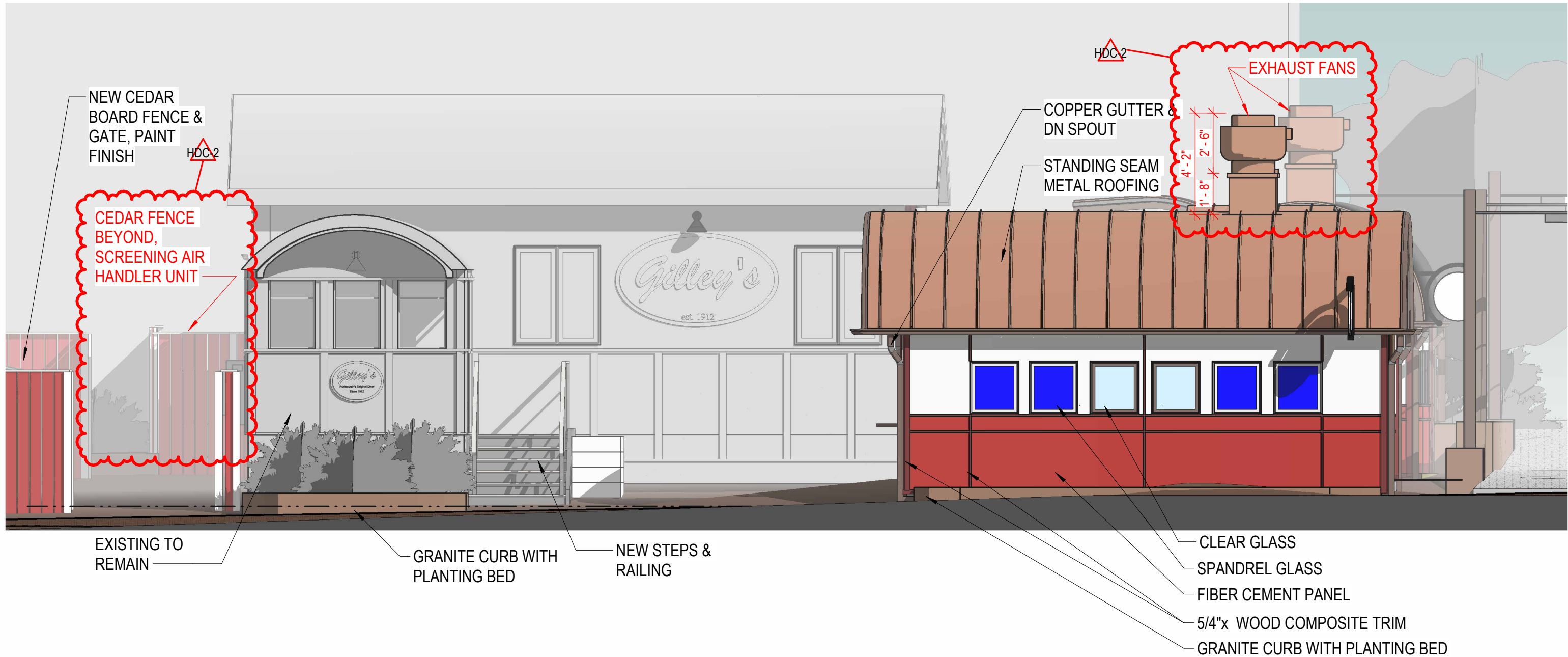
1 GILLEY'S WEST ELEVATION FLEET STREET VIEW 1/4" = 1'-0"
