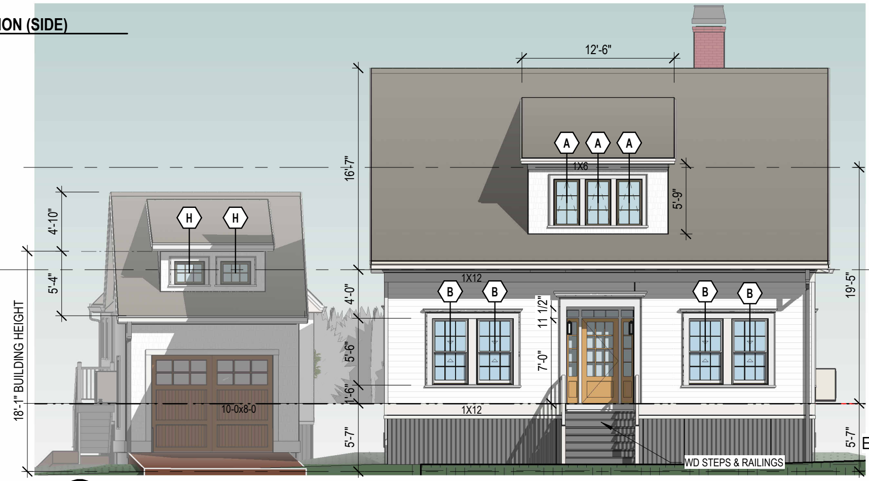
3 NORTH ELEVATION - PRAY ST (FRONT) 1/8" = 1'-0"
