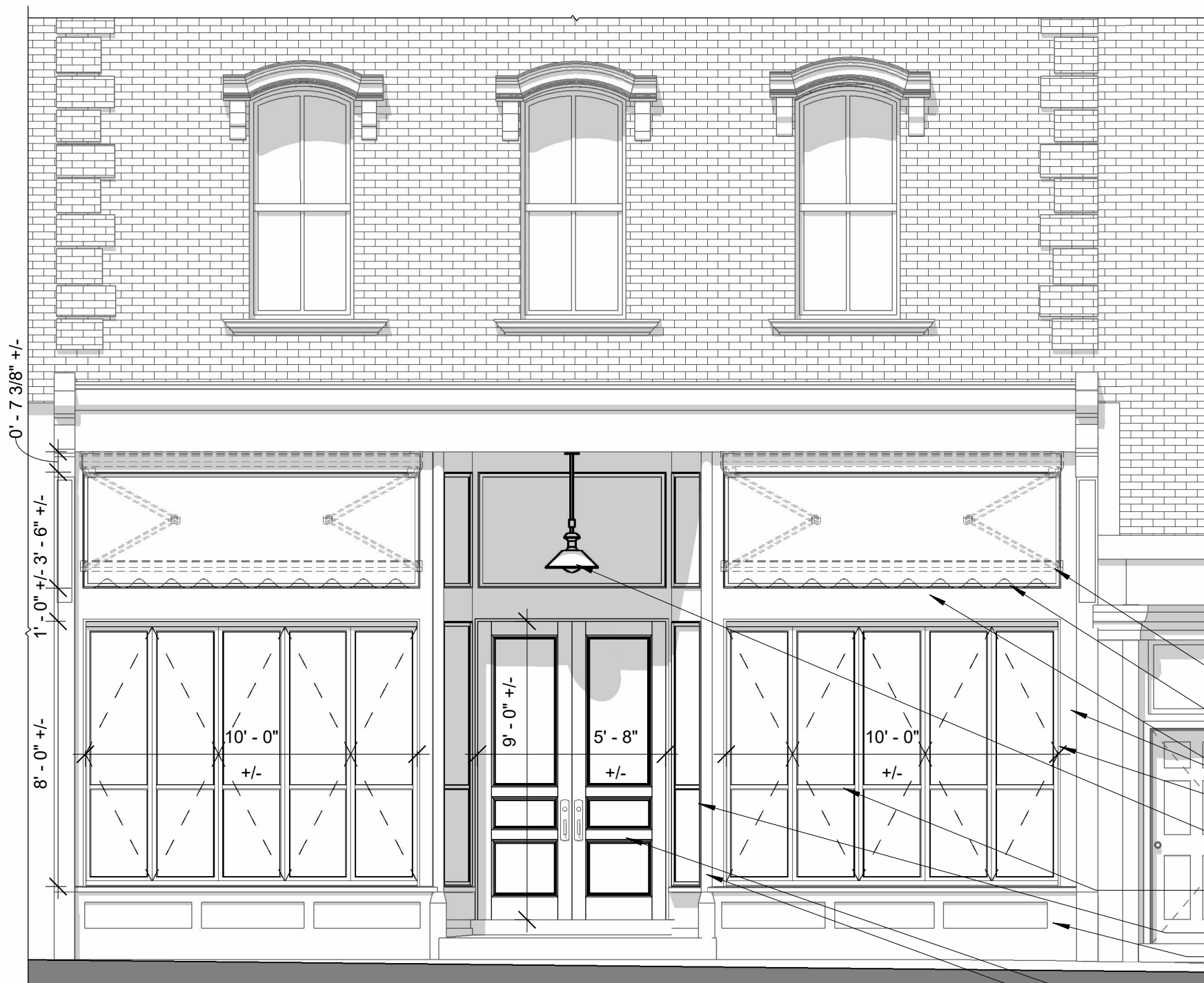
1 EAST ELEVATION AT STOREFRONT - OPTION 01 1/4" = 1'-0"
