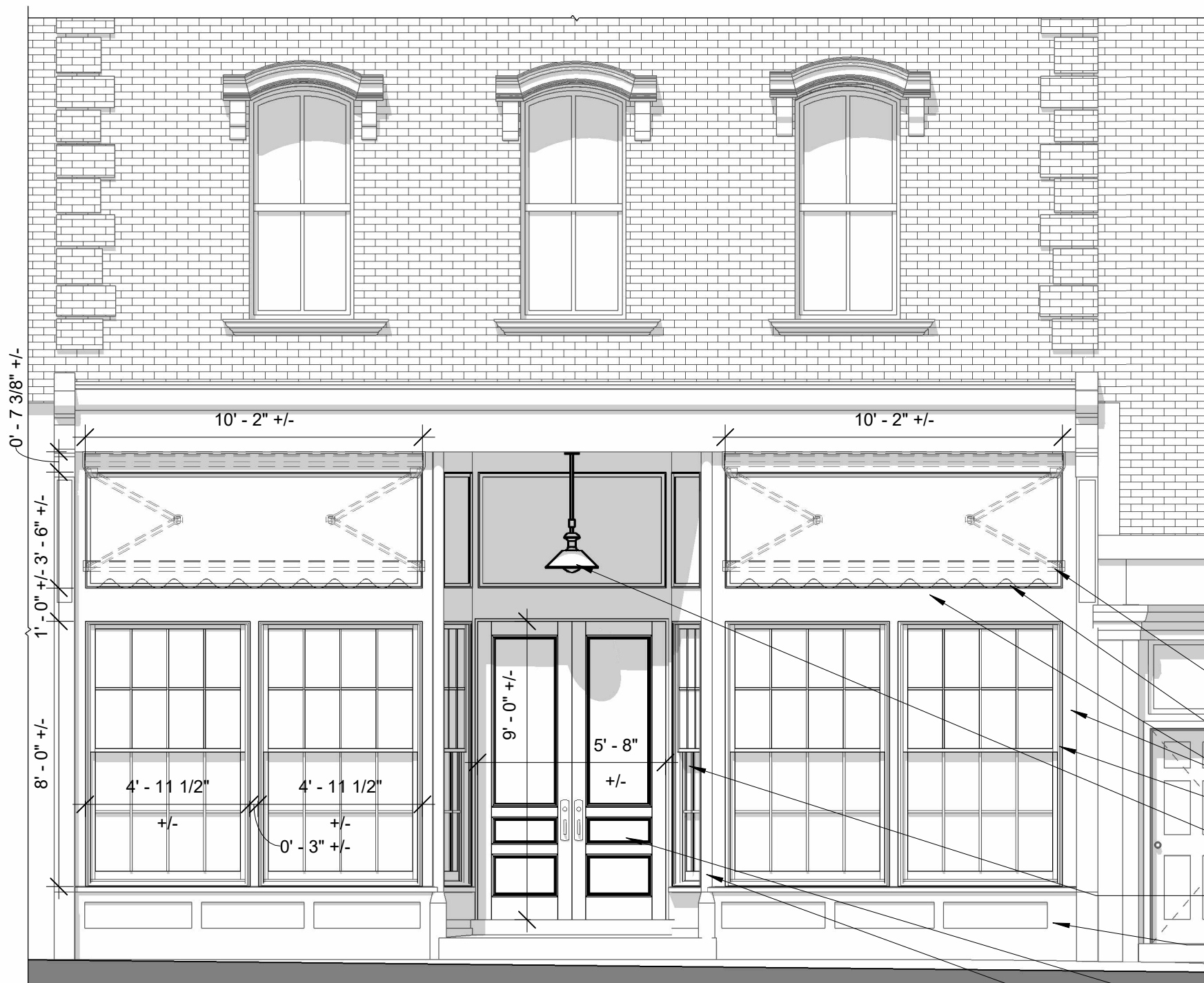
1 EAST ELEVATION AT STOREFRONT - OPTION 02 1/4" = 1'-0"
