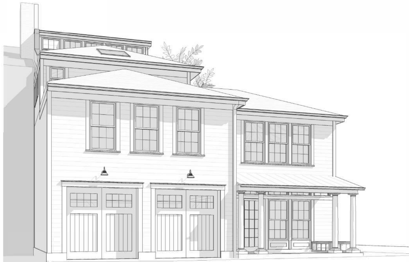
ALTERNATE - NO EAVE OVERHANG
